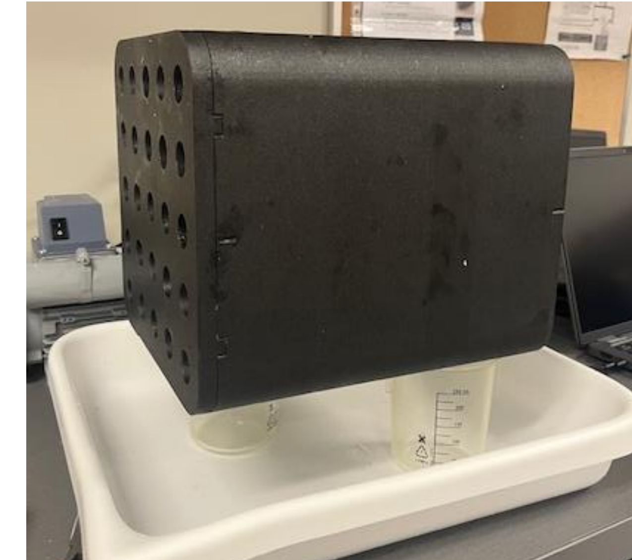
Figure 2 OPHELIA undergoing leak testing
