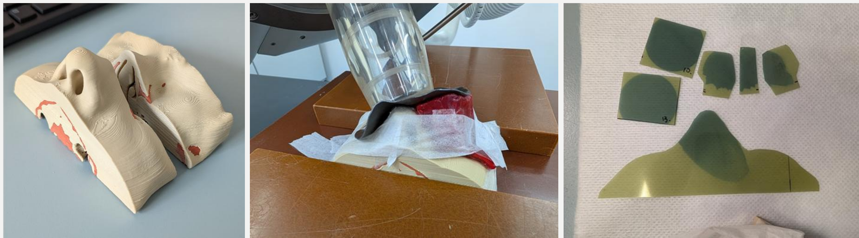
Figure 3. 3D-printed phantom, printed to facilitate film measurements using the Womed T-300 unit. Note that film has been placed on the surface of the phantom, as well as in a transverse plane between phantom pieces.
