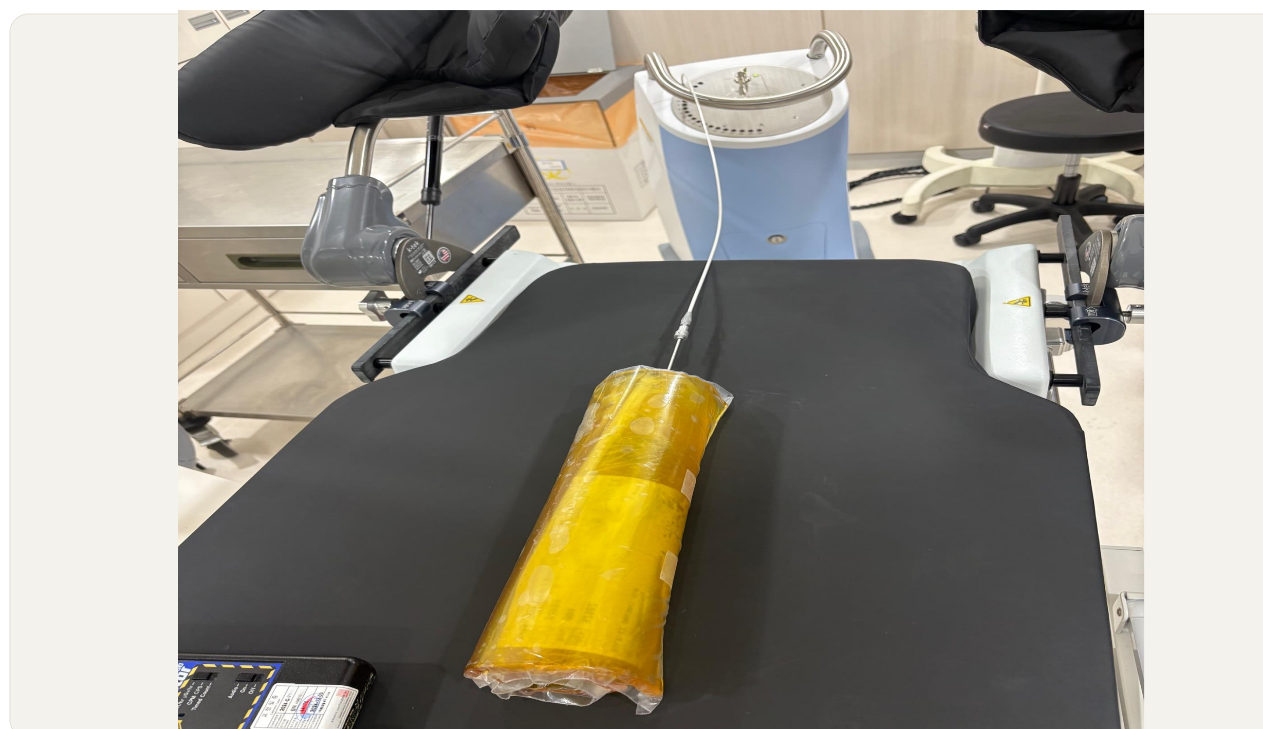
Figure 3. Experimental setup for TLD point dose measurement
