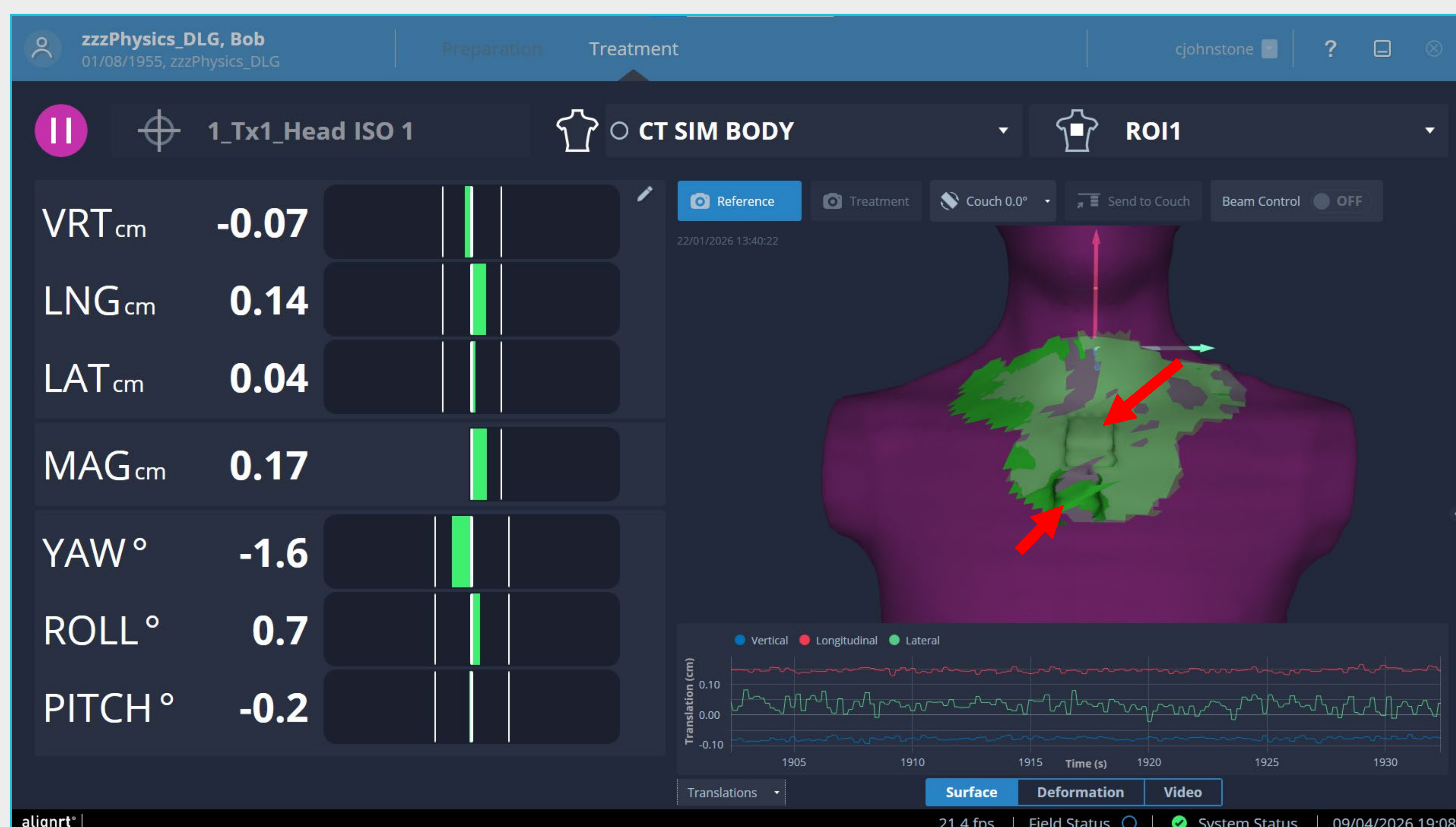
Figure 3: Using Surface Guidance with AlignRT to position the bolus on the Rando phantom. The top superior square within the Green ROI is the correct bolus position from the TPS, and the bottom inferior square is the real-time live positioning of the bolus. Correct bolus positioning is achieved when both bolus squares overlap.
