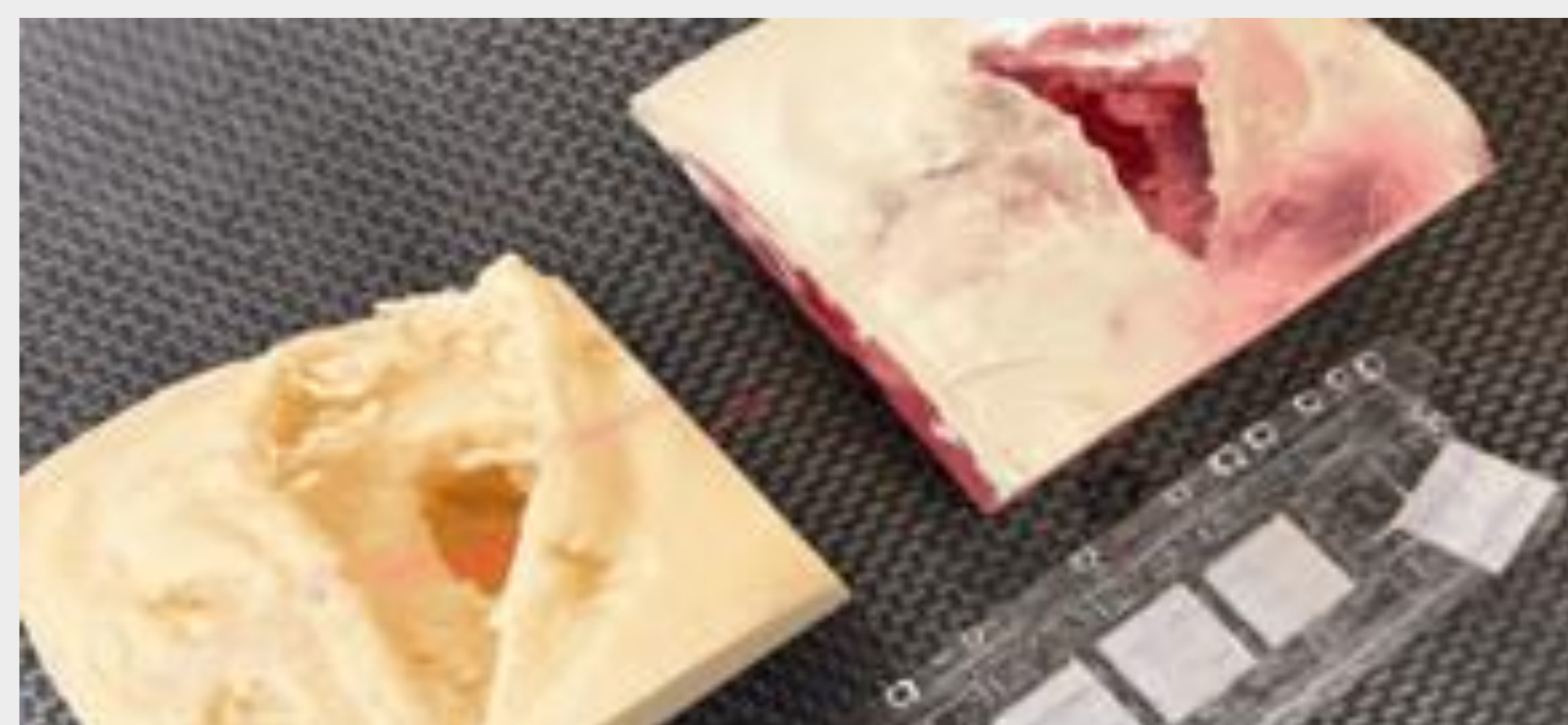
Figure 3. 3D-printed brain phantom with simulated resection cavity, used for ongoing imaging and workflow tests. Photo by researcher.
