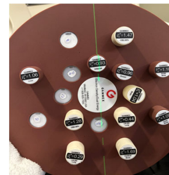
Figure 4. RMI phantom with inserts and vials containing \text{HfO}_2 solutions of various concentrations.
