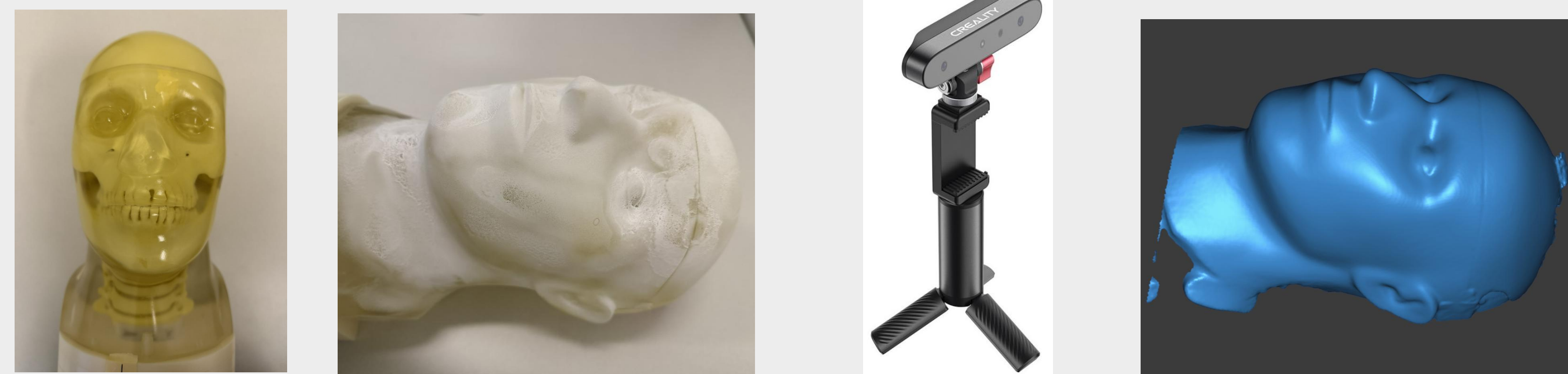
Figure 3. A hand-held 3D scanner and a head phantom used for surface acquisition. High-resolution 3D surface scan of the head phantom.
