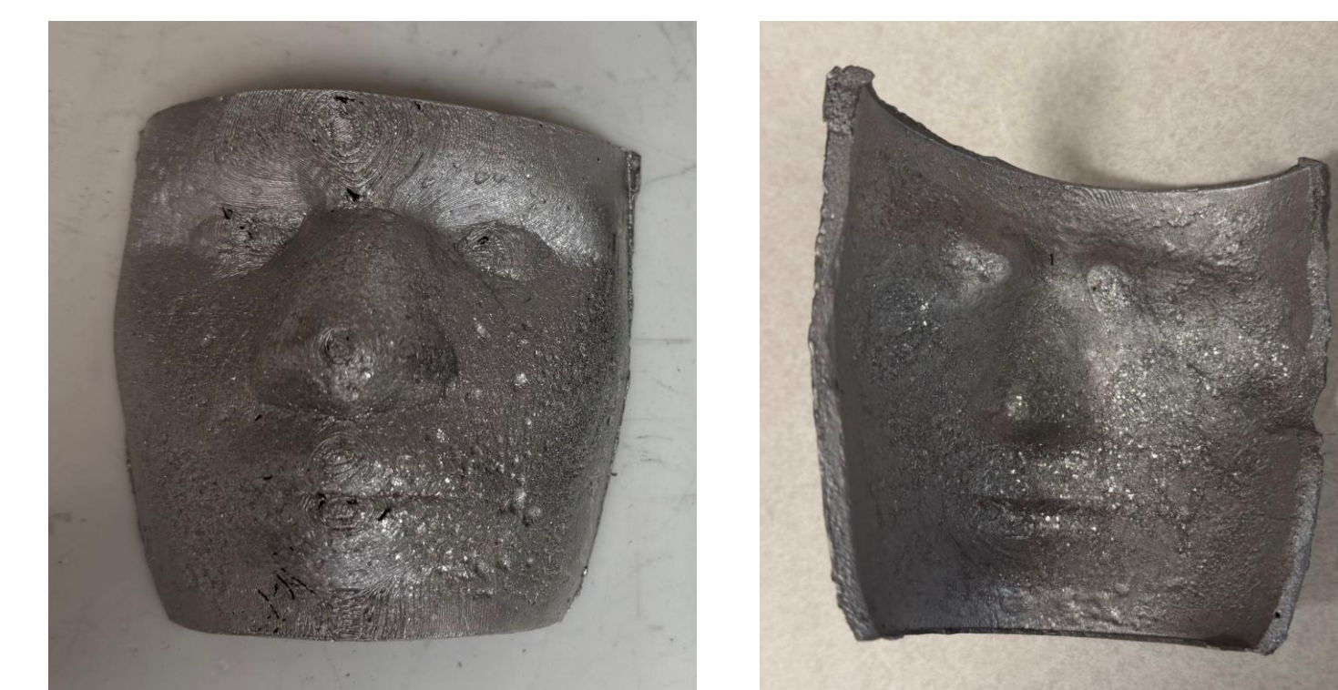
Figure 6. A prototype Cerrobend mask fabricated with 3D printed molds
