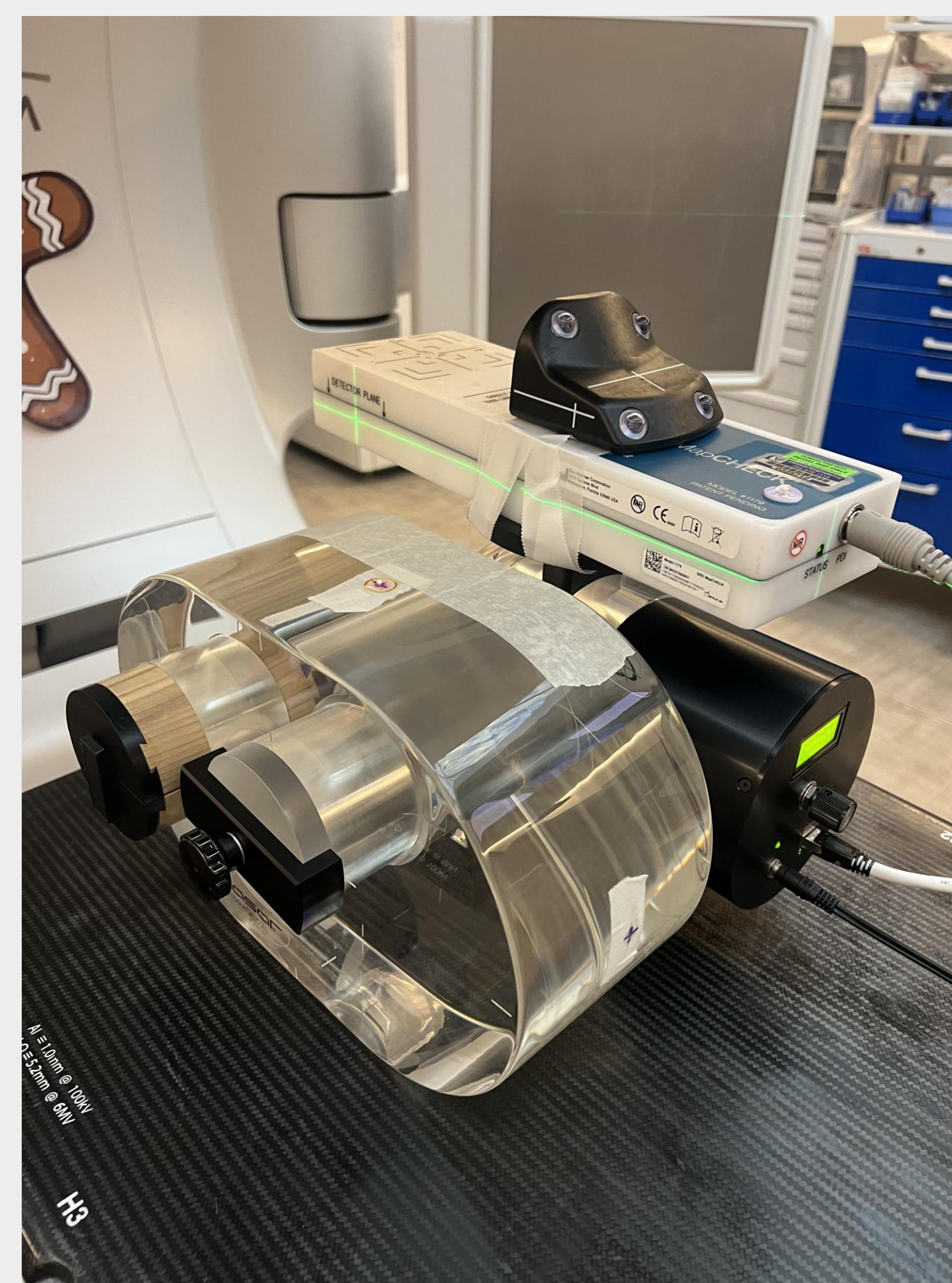
Figure 2. Quasar Modus Phantom setup with SRS MapCheck and RPM block
