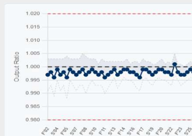
Figure 1. Per-event mean output ratio ( \pm 1 SD) over 46 semiannual intercomparison events, 2002–2026. Dashed lines indicate \pm 2\% action levels.
