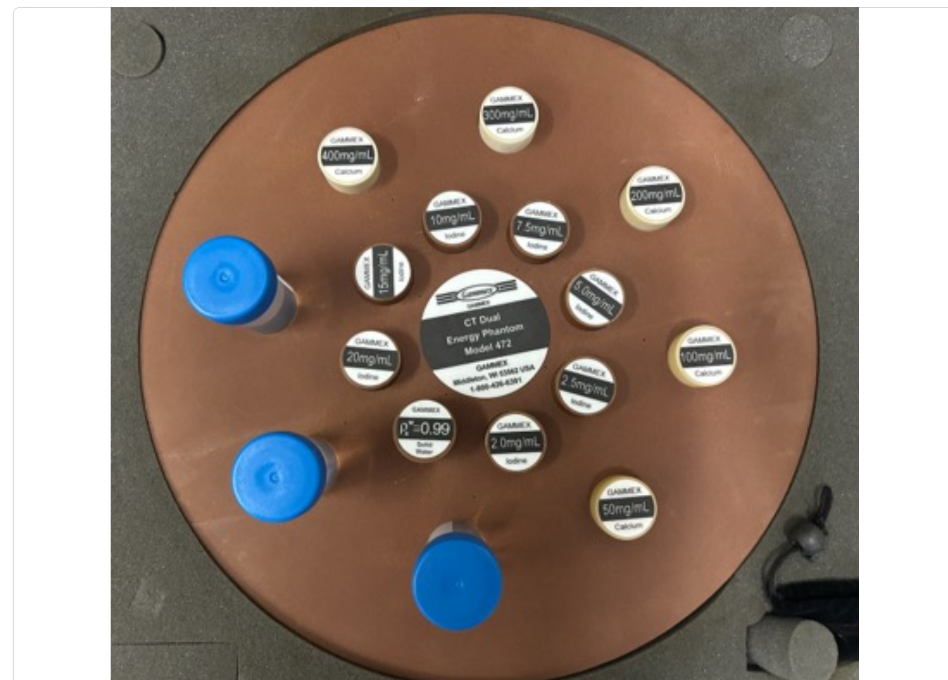
Figure 2. Physical Gammex 472 phantom used for the experimental acquisition.
