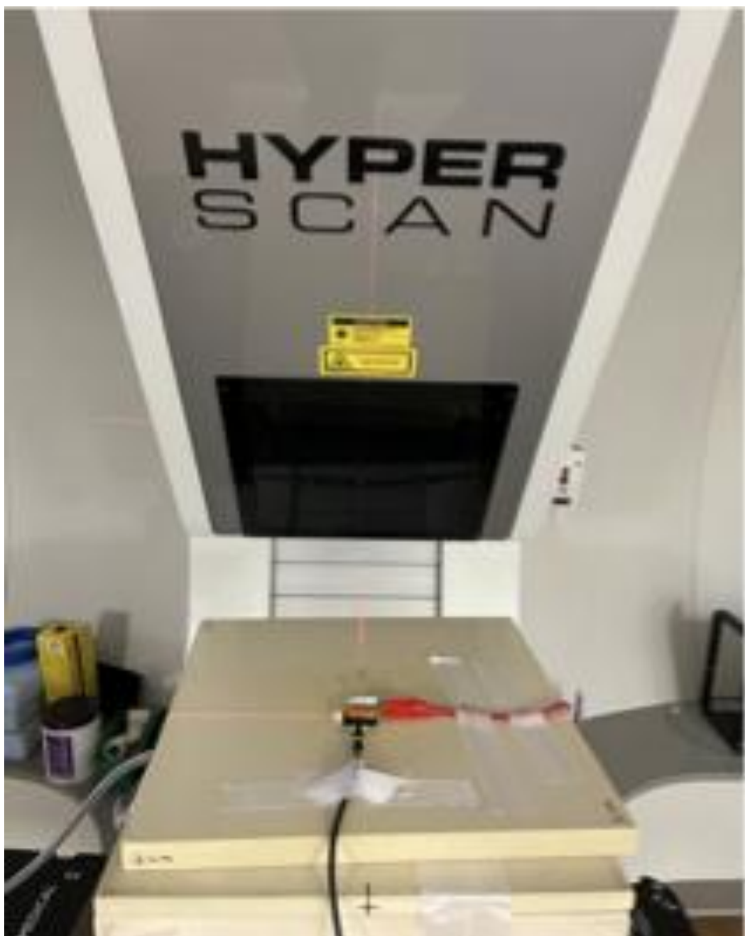
Figure 1. Experimental setup for proton irradiation. A single-spot proton beam from the Mevion HYPERSCAN S250i system was used to irradiate the detector. Before the experiment, the surface dose at the detector position was independently calculated using the treatment planning system (TPS) and Monte Carlo (MC) simulations.
