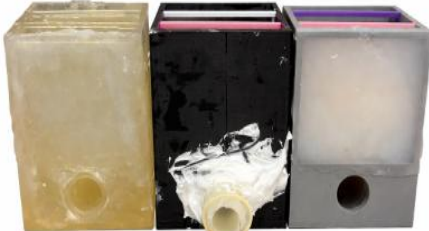
Figure 2: Transverse photograph of phantom boxes housing synthetic gel, water, and agar, respectively.
