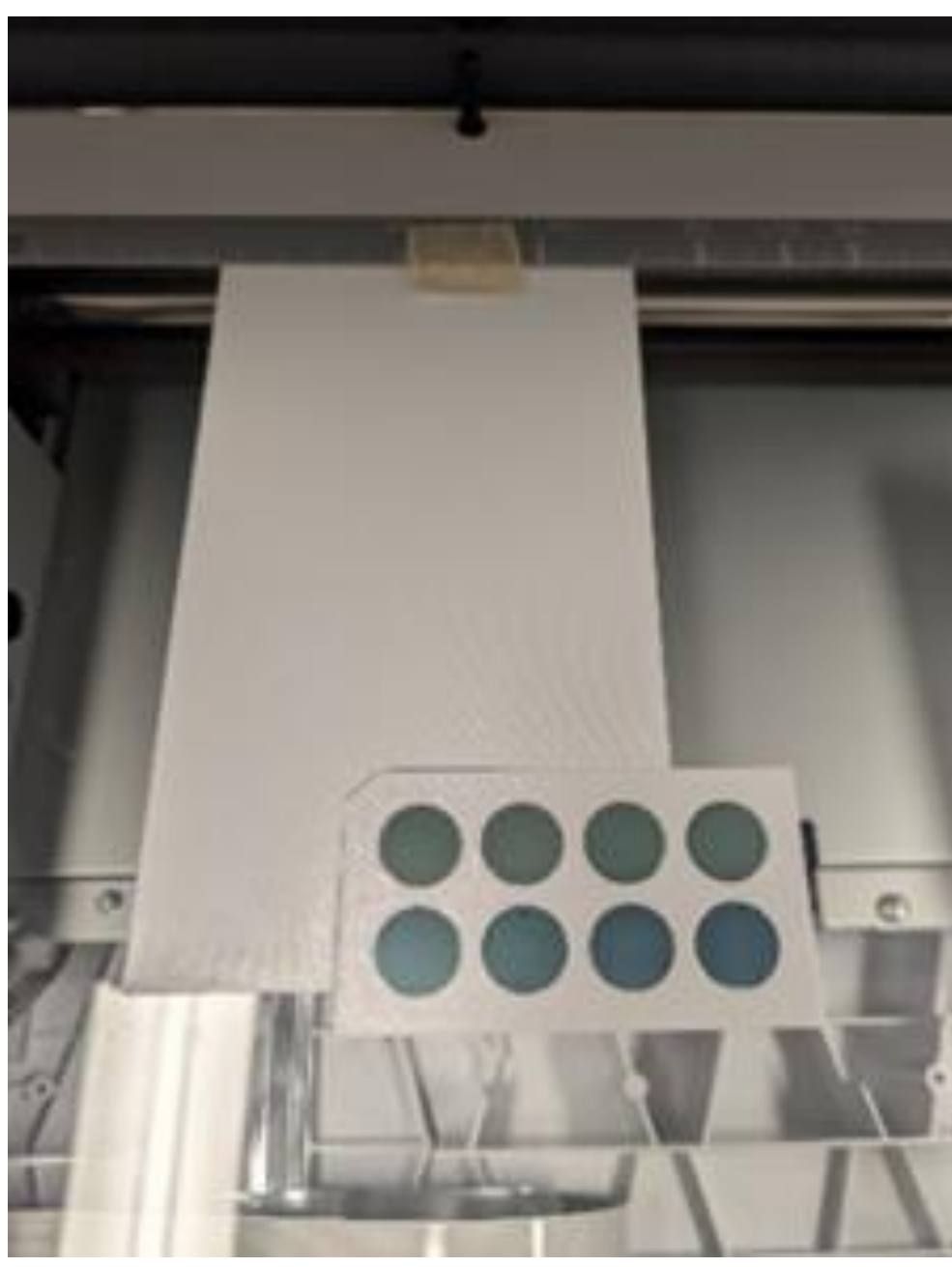
Figure 2. An EPSON 12000XL flatbed scanner was used to create calibration curves. A 3D-printed holder was used to ensure reproducible film positioning.
