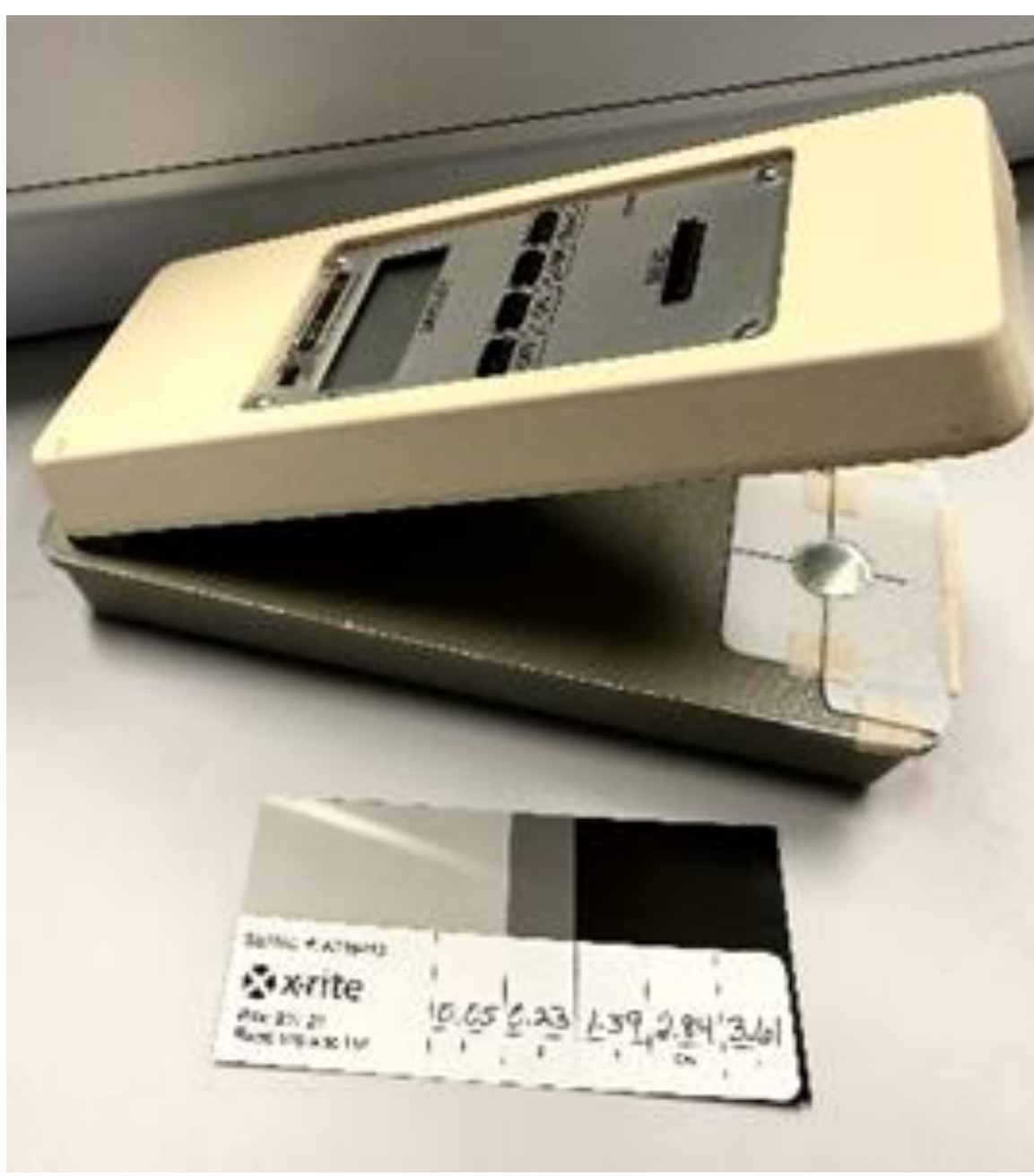
Figure 3. An X-rite Model 331 transmission densitometer was used to create a calibration curve. The X-Rite Model 331 transmission densitometer was calibrated using the manufacturer's calibration strip.
