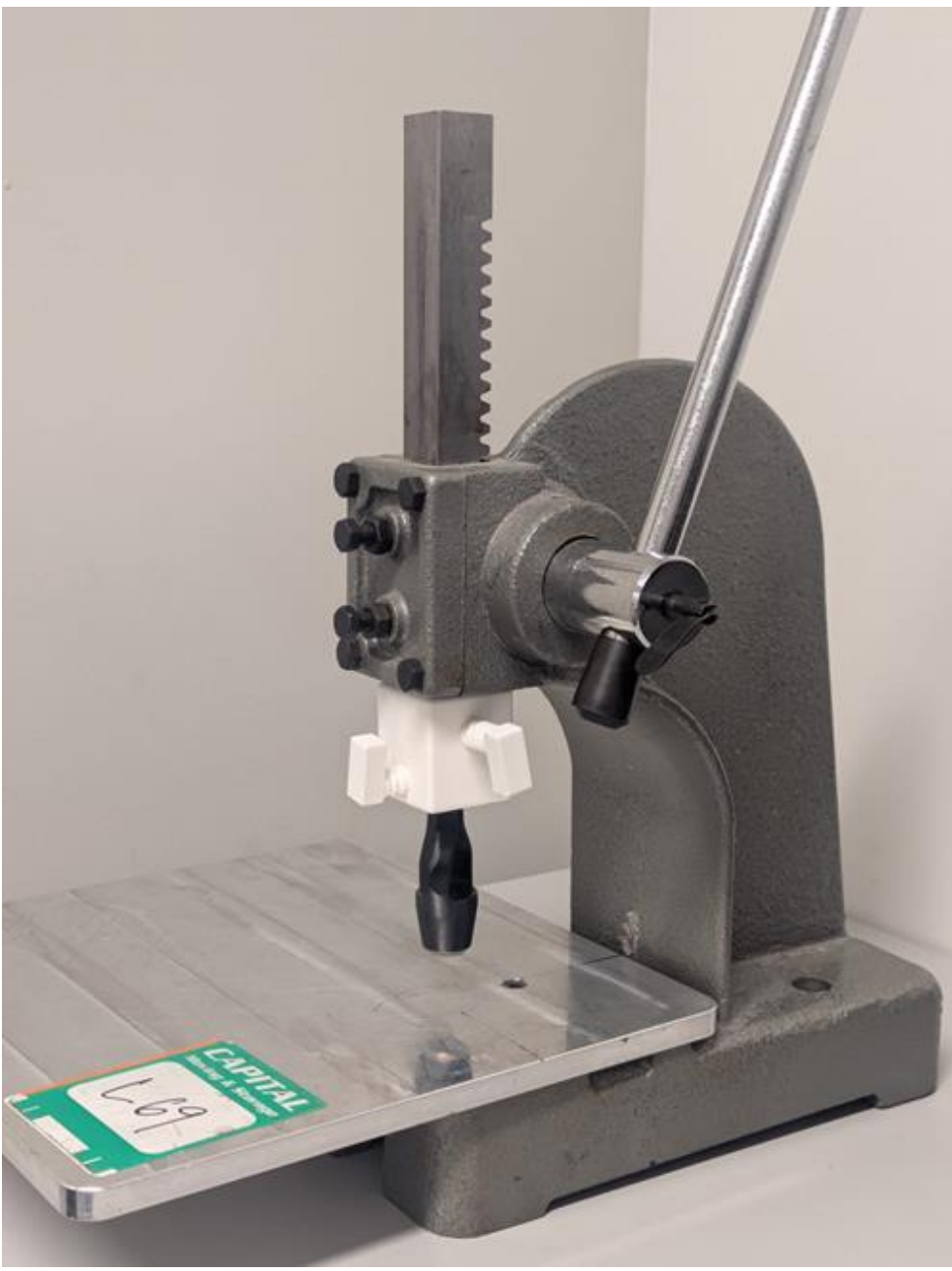
Figure 1. Using an arbor press and arch punch, 16-mm discs were cut from sheets of EBT4 film and calibrated in solid water using 6 MV photons.
