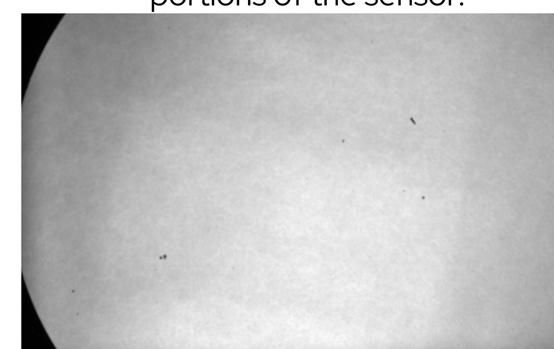
Example of a flatfield image where the light intensity imaged by the sensor falls off at the periphery
