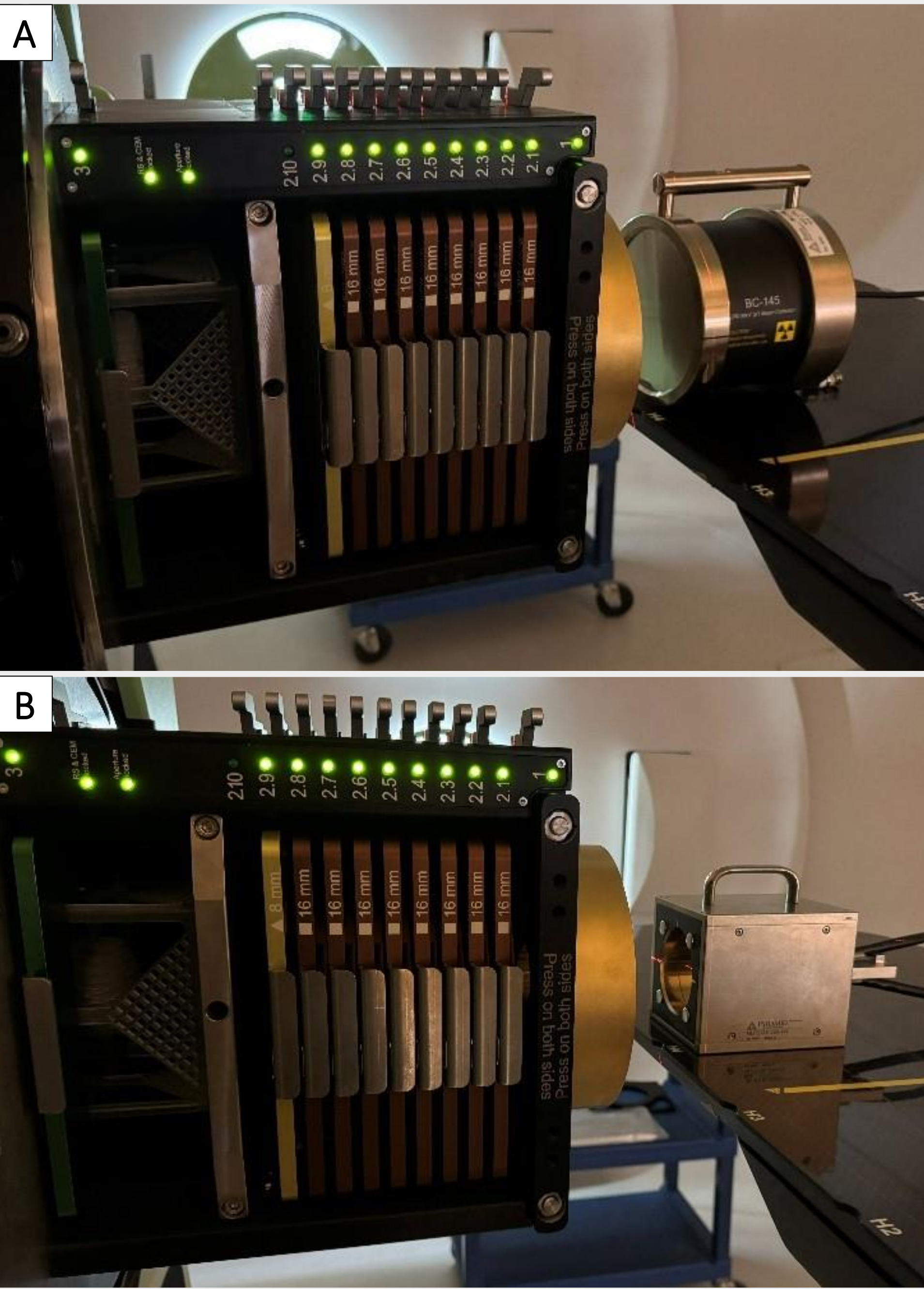
Figure 1: Experimental setup of the A) Faraday cup (FC) and B) multi-layer Faraday cup (MLFC) for UHDR proton PBS FLASH beam characterization. The scanning beam passes through energy-modifying components in a conformal FLASH nozzle before charge collection.
