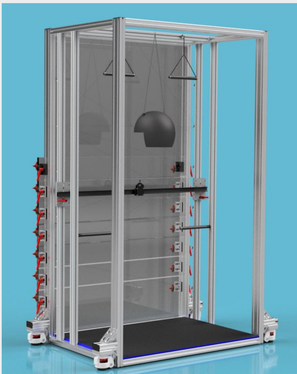
Figure 2: CAD Rendering of TSET Frame, Helmet, and QA Rail
