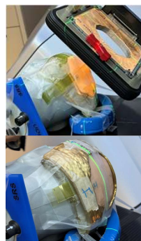
Figure 2. The setup of phantom study and in-vivo dosimetry. Upper left: phantom study without brass surface collimation. Lower left: phantom study with brass surface collimation. Right: In-vivo dosimetry setup with patient in prone position. The film strip was placed in SI-direction. The field edge was marked on the film for further comparison and analysis. In addition, the film was placed partially underneath the silicon bolus and partially underneath the brass collimation.
