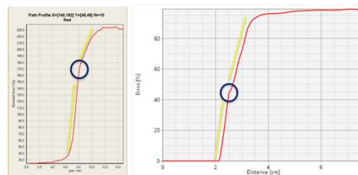
Figure 3. Film profile from in-vivo dosimetry (left) and the dose profile reported from treatment planning system (right).
