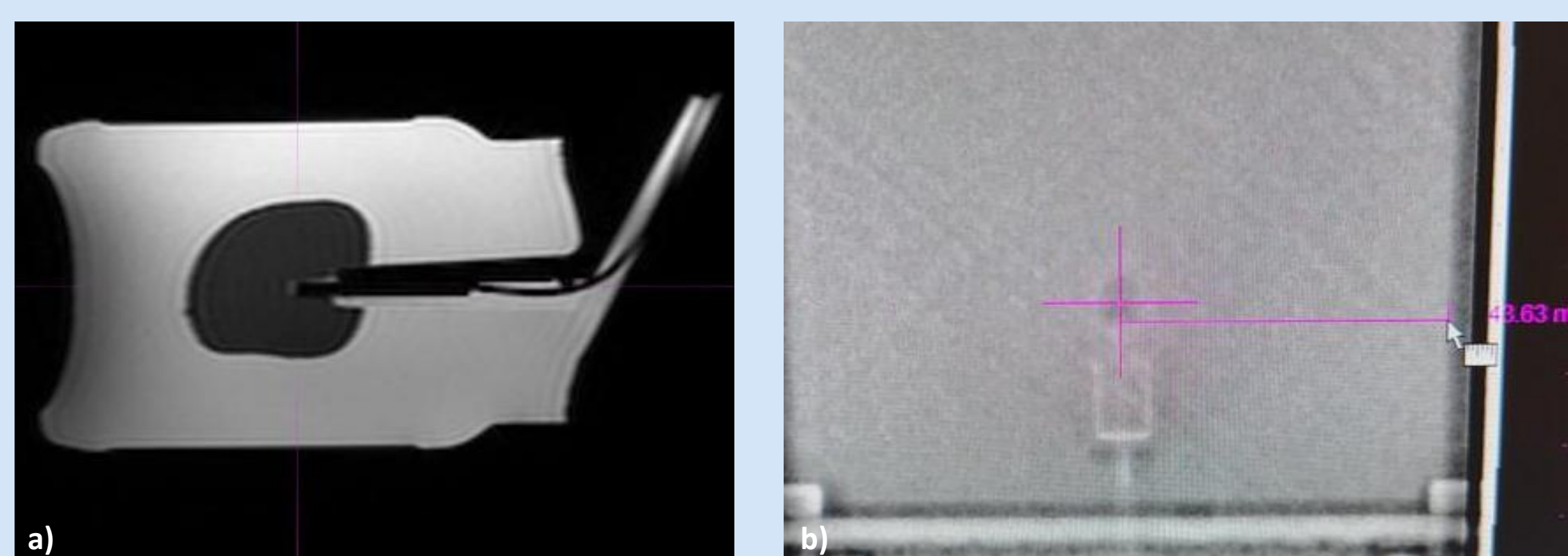
Figure 4. : a) T2-weighted image from the MR-Linac of the PSD inside the silicone insert b) MR-Linac portal verification image of the phantom with the CC13. The cross hair shows the machine imaging isocenter
