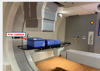
Figure 1. Conventional PSQA setup at 0 degrees, with added solid water build up.
