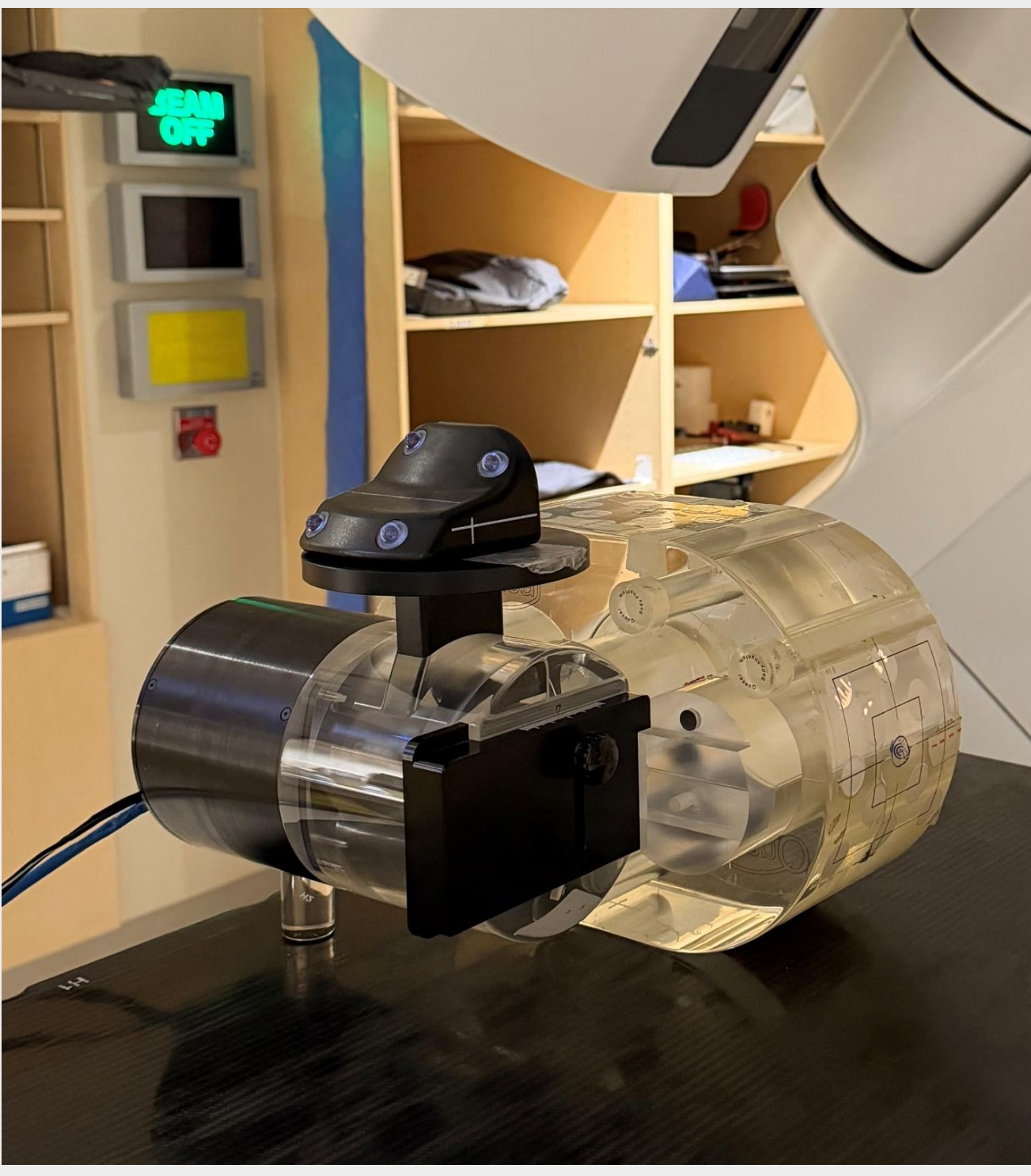
Figure 2. Film dosimetry setup with Quasar pRESP phantom and Varian marker block.
