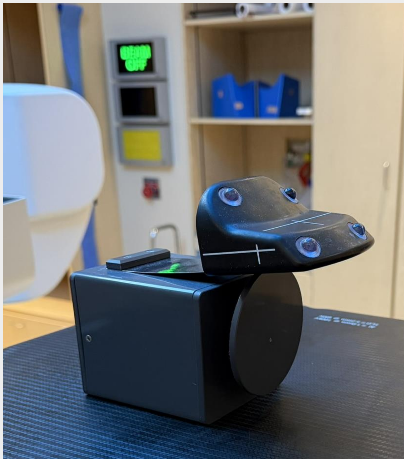
Figure 1. Portal dosimetry setup with Varian motion phantom and marker block.
