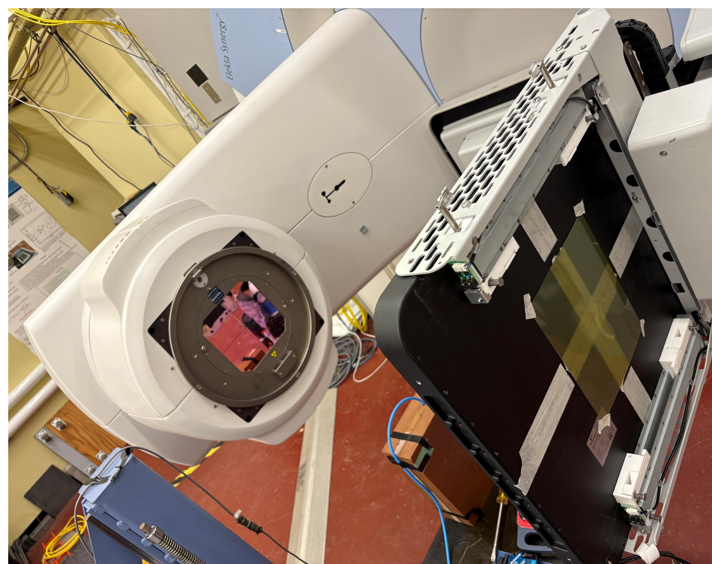
Figure 3: In-EPID film measurements set up showing the film on the back cover
