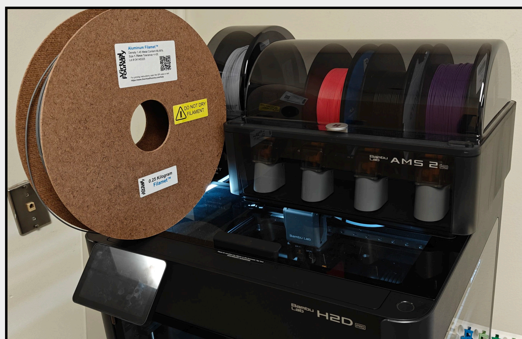
Figure 1. Aluminum 6061 Filamet™ from Virtual Foundry, Inc., printed using the Bambu Labs H2D Pro dual nozzle printer.
