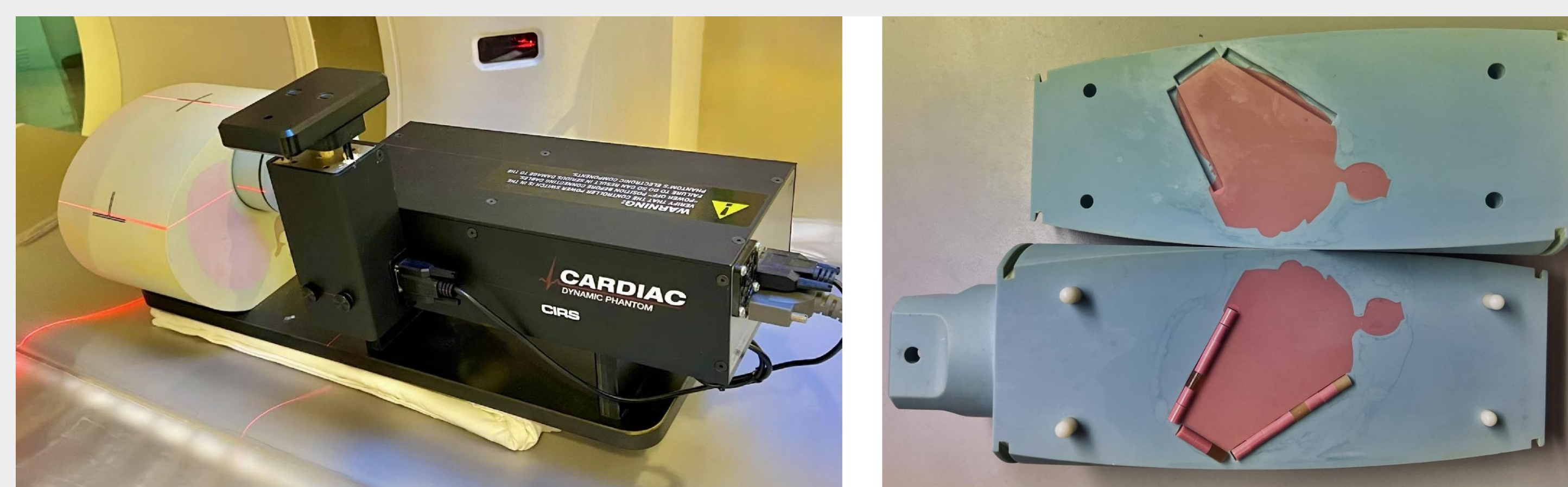
Figure 1. Dynamic cardiac phantom. (A) Phantom placement inside CT gantry. The actuator was driven by a motion controller in the back. (B) Two phantom halves with a 13° split angle and a coronary artery track.
