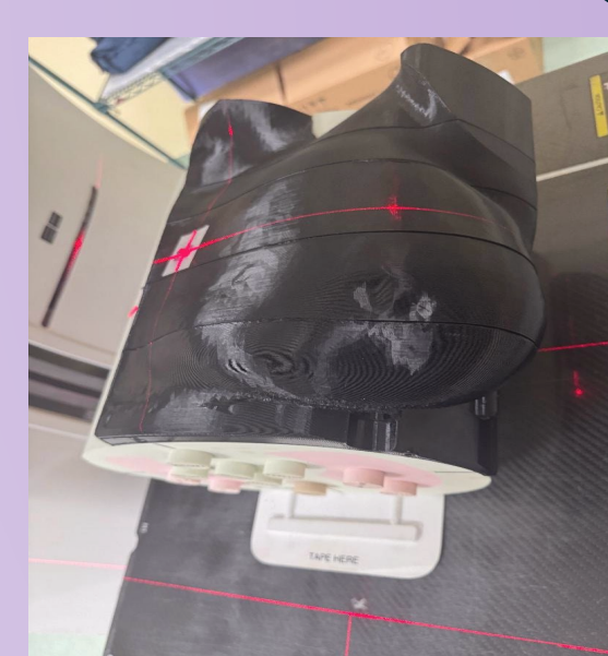
Figure 12: CT Scan Setup of BRENDA- Breast and Regional Lymph Node End-to-End Dosimetry Assessor
