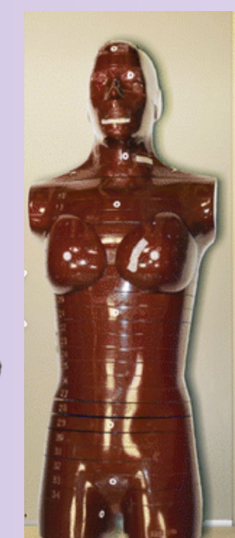
Figure 5: Alderson Radiation Therapy (ART) Phantom
