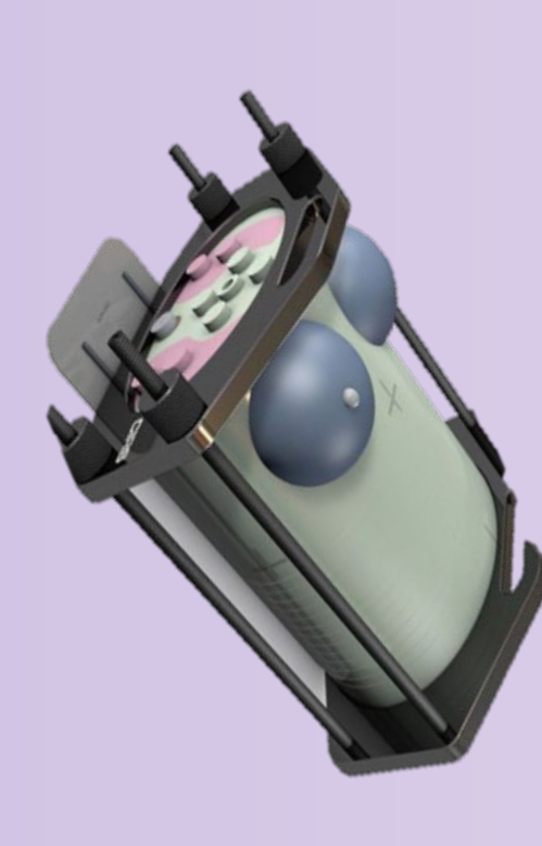
Figure 4: CIRS IMRT Thorax Phantom with breast attachments
