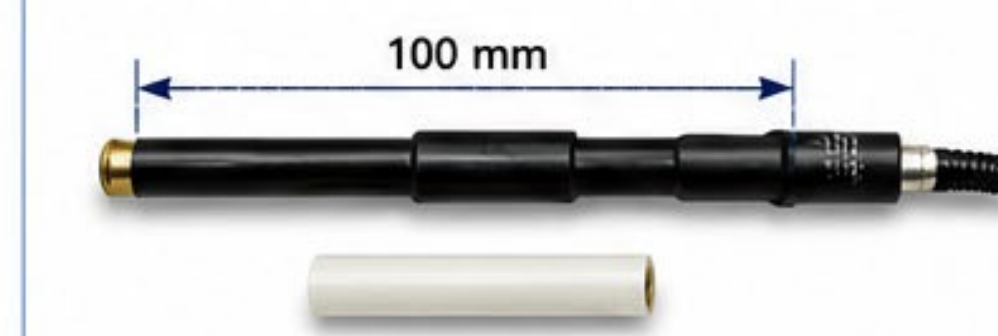
Figure 1. Standard CTDI phantoms and 100-mm pencil ionization chamber used for CT dose measurements. A 16-cm diameter head phantom and a 32-cm diameter body phantom composed of polymethyl methacrylate (PMMA) were used to perform CTDI measurements following the standard CTDI methodology. A calibrated 100-mm pencil ionization chamber was inserted into the phantom measurement holes to acquire CTDI data.
