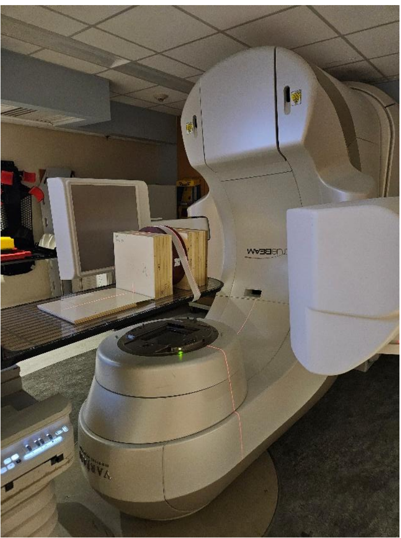
Fig 1: TrueBeam Calibration setup (Left) utilizing Gammex model 467 plug phantom (Middle). 125 kVp image shown (Right) containing high density core and titanium plugs and tissue plugs ranging from 0.28 to 1.69 relative electron densities.
