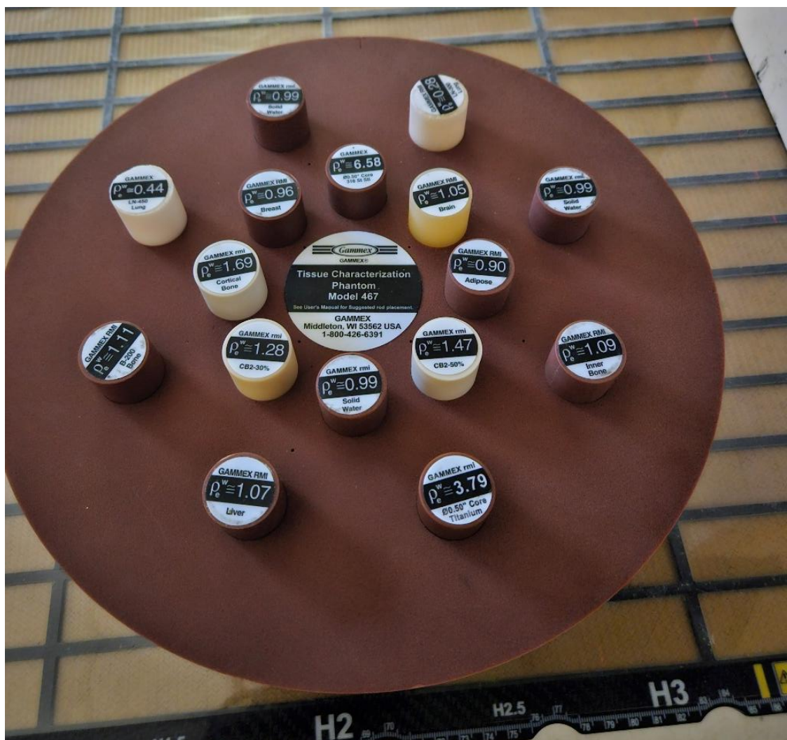
Fig 1: TrueBeam Calibration setup (Left) utilizing Gammex model 467 plug phantom (Middle). 125 kVp image shown (Right) containing high density core and titanium plugs and tissue plugs ranging from 0.28 to 1.69 relative electron densities.
