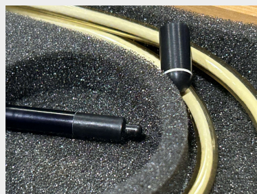
Figure 2. Exradin A16 pinpoint chamber 0.007cc collection volume. 1mm diameter equivalent.
