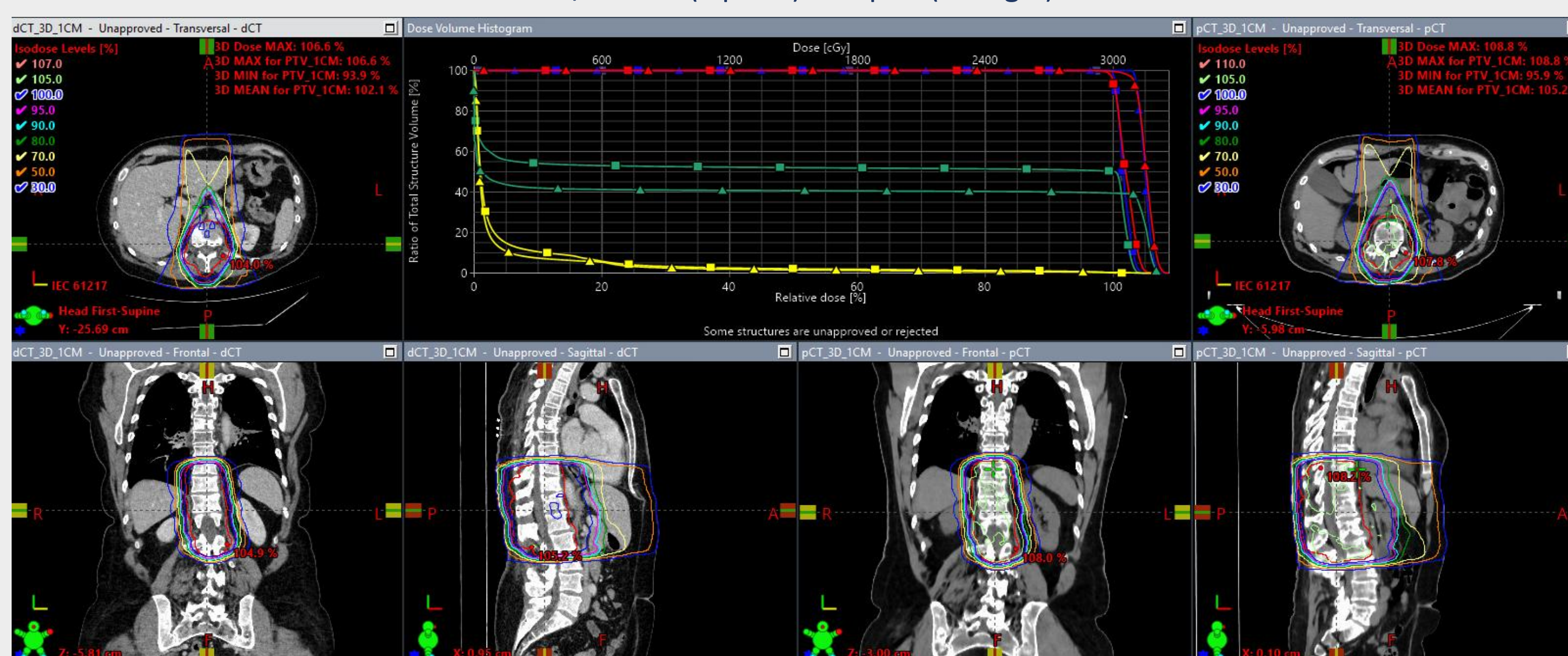
Figure 3. DVH comparison of the PTV (red), CTV (blue), lungs (yellow), and spinal cord (green) of one patient's 3DCRT dCT (square) and pCT (triangle).
