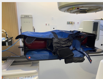
Figure 2. Anthropomorphic phantom with ionization chamber and lead Configuration. This figure includes 1 anterior + 1 posterior lead apron
