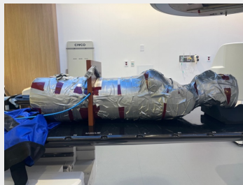
Figure 1. Anthropomorphic Phantom with ionization chamber setup.
