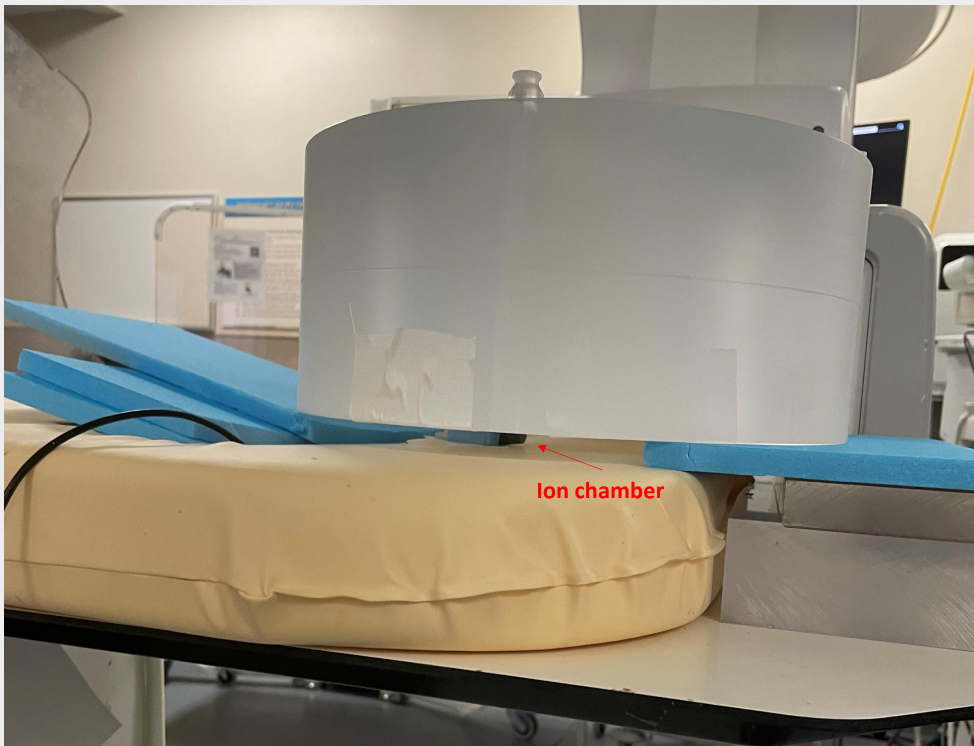
Figure 1. 32-cm CTDI phantom supported by Styrofoam blocks and just touching the ion chamber on the uncompressed pad.
