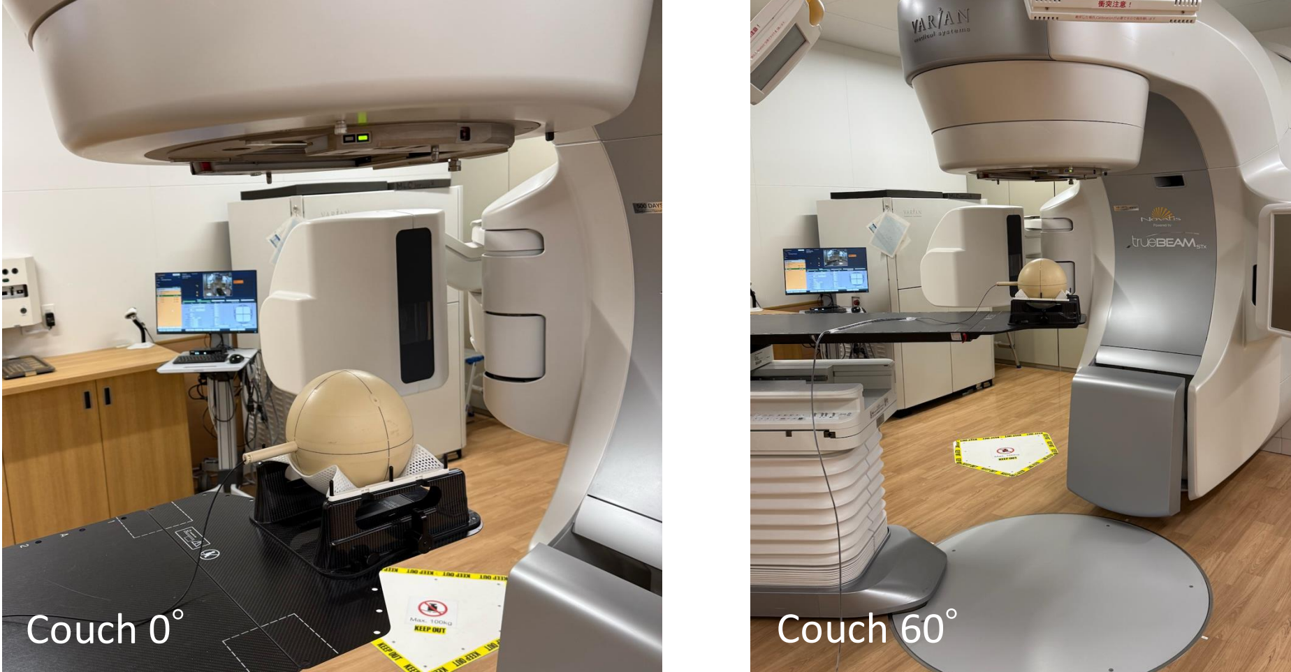
Figure 2. Non-coplanar arc setup at couch angles of 0^\circ (left) and 60^\circ (right). Couch angle determines the beam–fiber geometry; during arc delivery, gantry rotation changes the volume of transport optical fiber irradiated by the beam, thereby altering the Cherenkov contribution.
