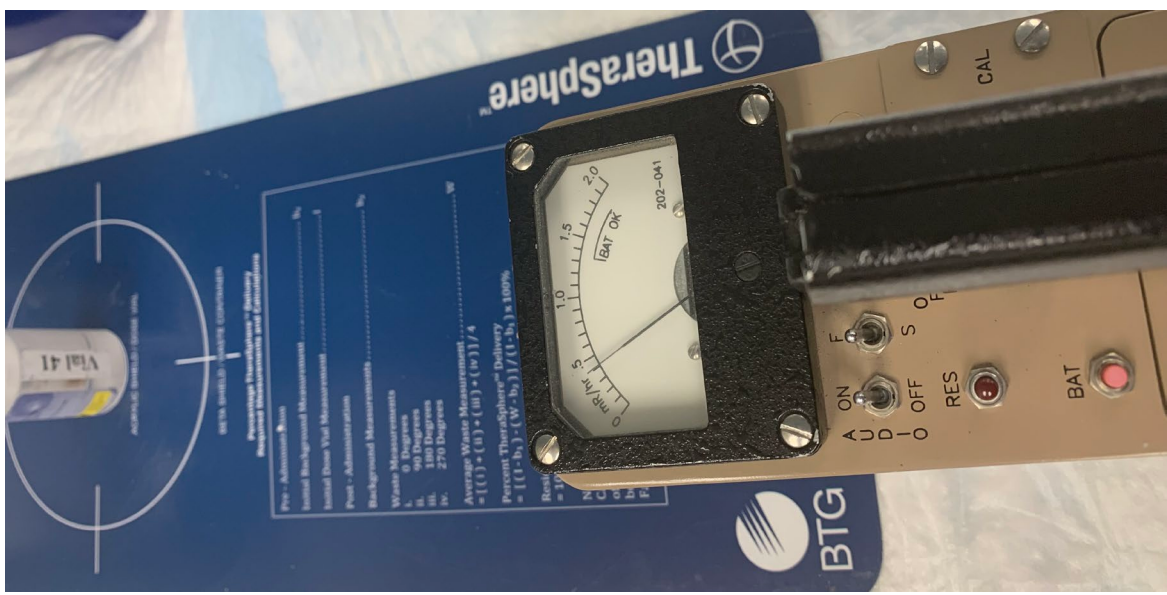
Initial exposure rate reading with uncertainty: E \pm (\Delta E + S \times E)
