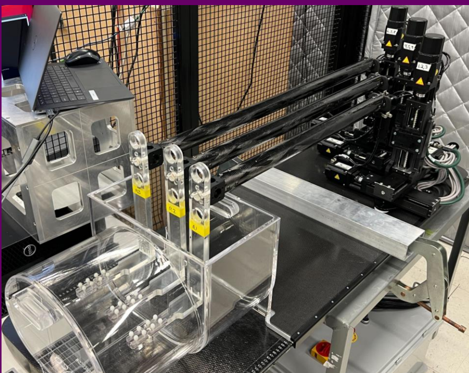
Custom water-filled phantom with independently moving arms
