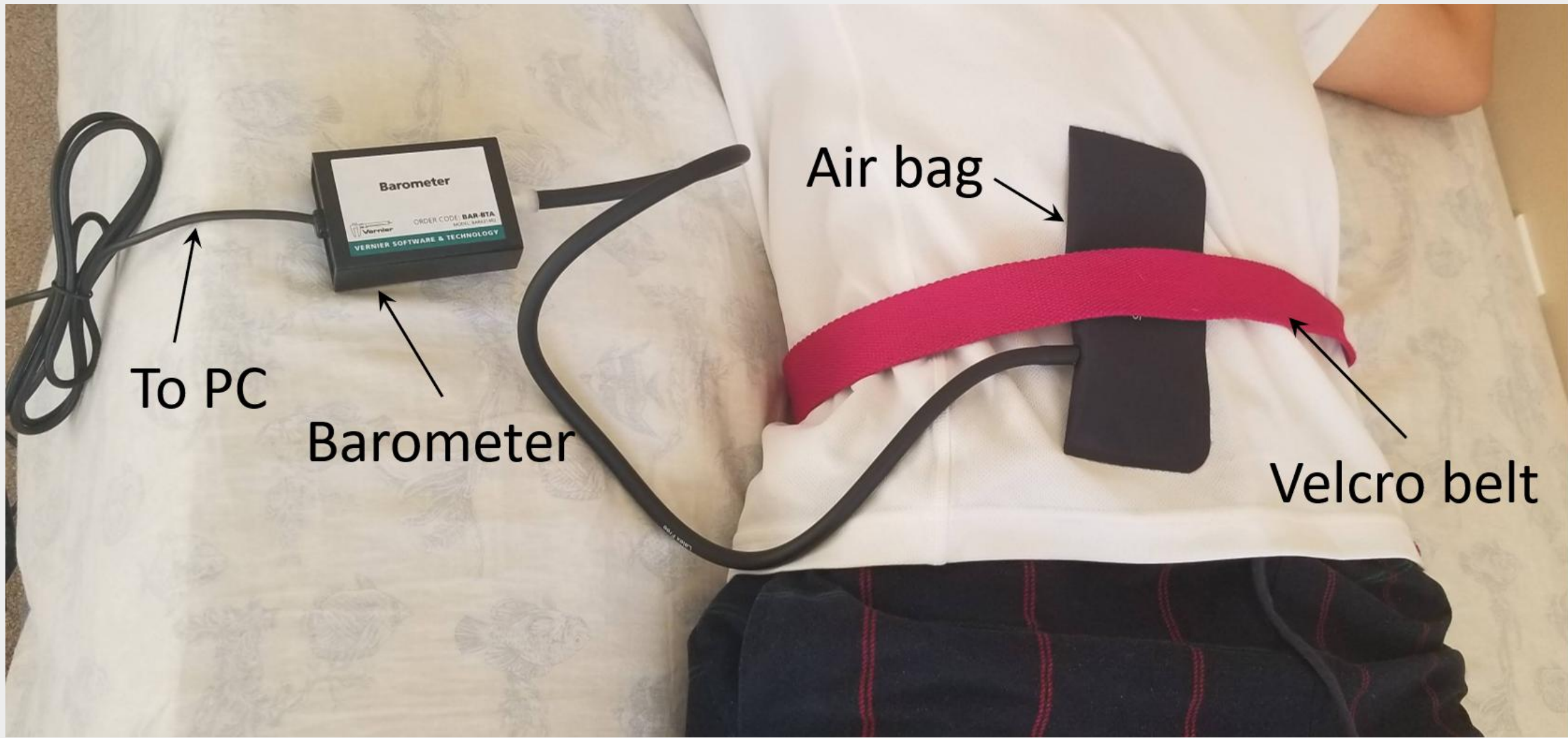
Figure 2. In-House Monitoring Hardware. The custom in-house respiratory monitoring system utilizes an air pressure sensor to measure and display these breathing patterns to bridge the technical gap during the MRI acquisition phase.
