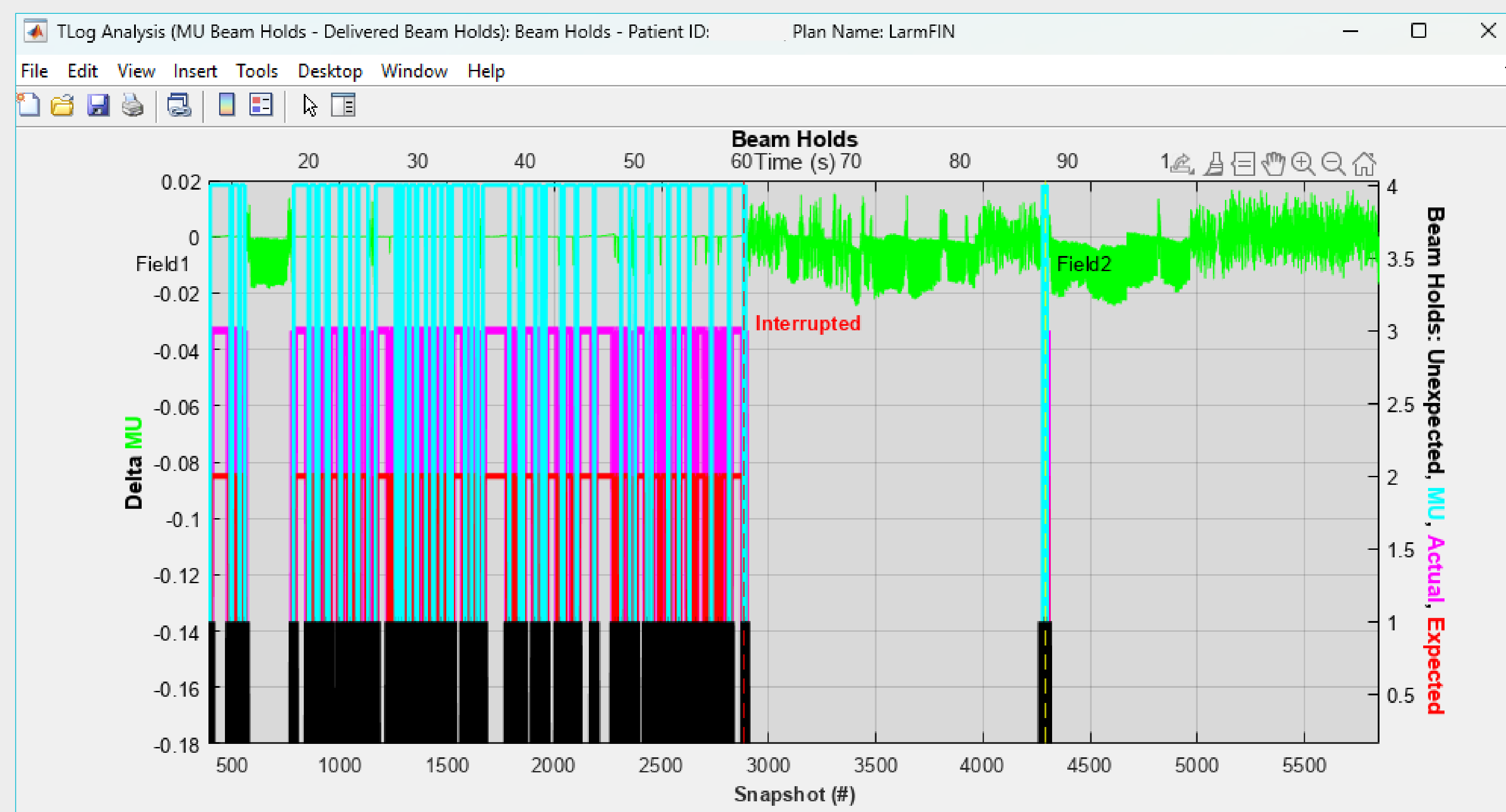
Figure 3: Illustration of excessive unexpected beam holds during the first field leading up to a treatment interrupt. Displayed are actual (delivered), expected (TPS), MU (MUs don't increment), and unexpected (actual minus MU) beam holds. Unexpected beam holds may be an indicator of mechanical delivery problems.
