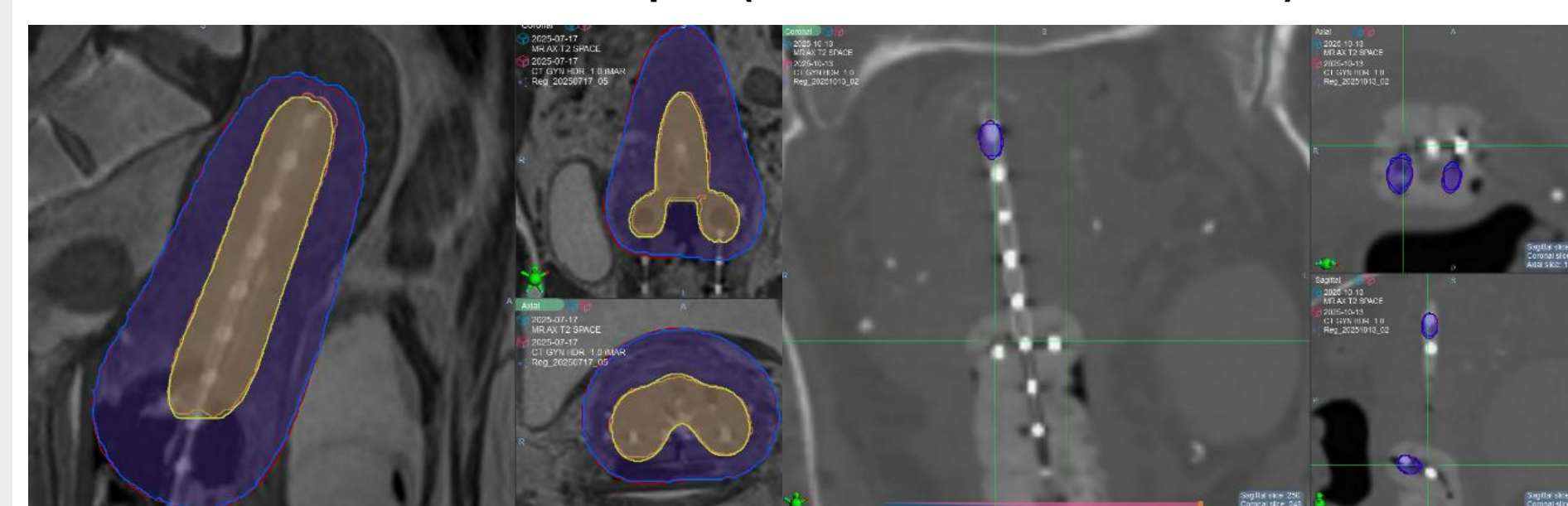
Screenshot above shows the 100% and 250% IDLs on CT and MRI superimposed on each other. Blue-100%IDL on CT; Red - 100%IDL on MRI; Orange-250%IDL on CT; Yellow-250%IDL on MRI.
