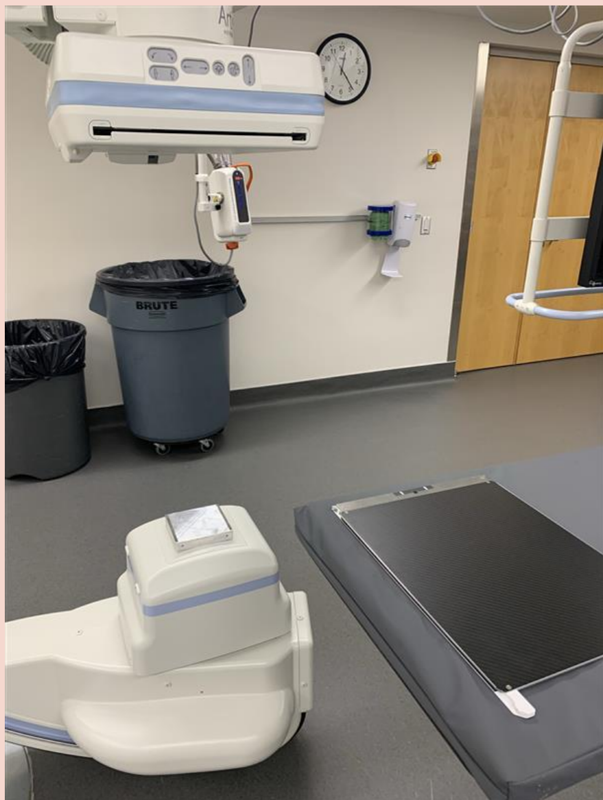
Figure 1. Flat-field image setup with RQA5 phantom and detector grid removed.
