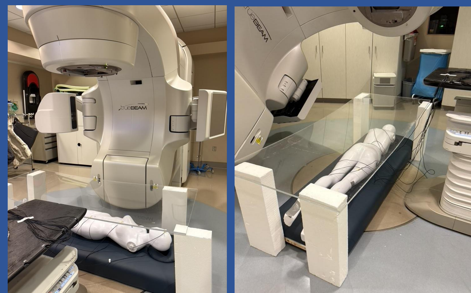
Figure 5. Irradiation of homogeneous anthropomorphic phantom with diodes. Supine position (left). Prone position (right).
