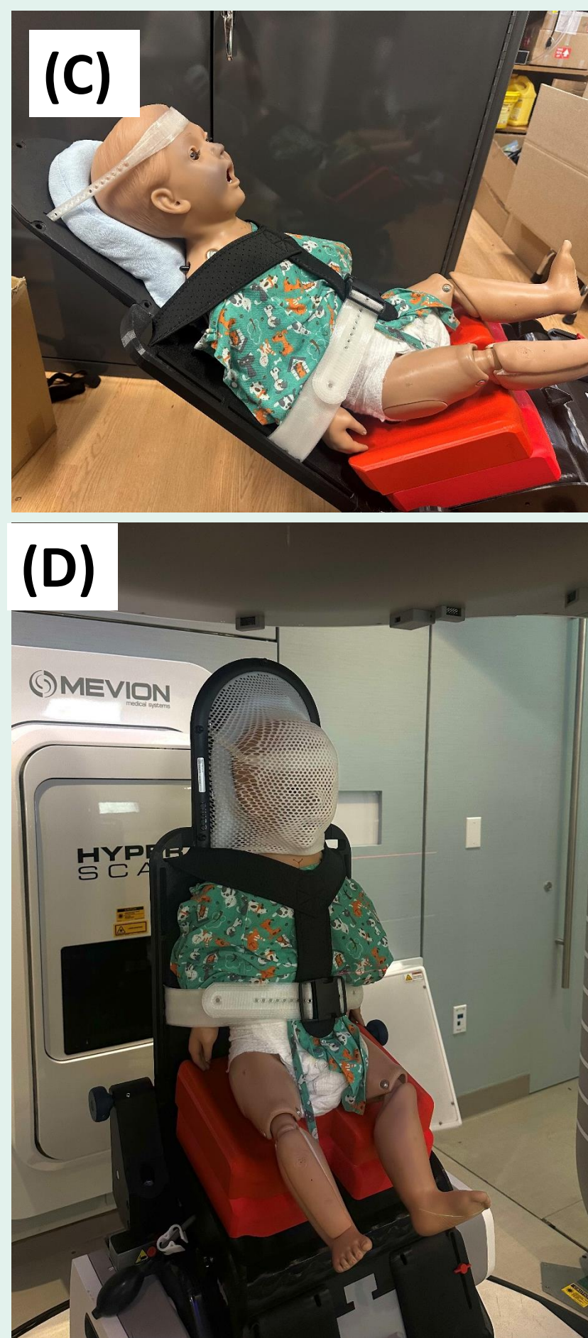
Figure 2. A) 3D diagram of chair design (external and internal components). B) 3D printed chair mounted on Leo chair system. Note 5cm boosters stacked, knee fix at top, waist belt and Velcro cross-body straps. C) Phantom in induction position with straps and Accuform. D) Phantom with mask and straps in upright position.
