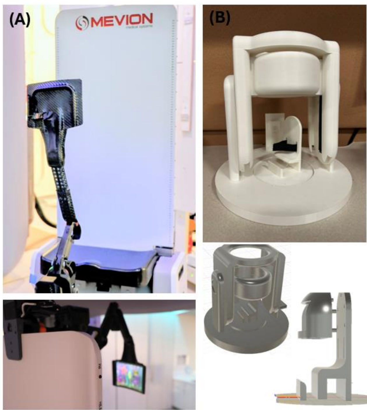
Figure 4. A) AVATAR system modified to fit upright chair setting. B) 3D model of upright Leo CT and chair for pediatric familiarization.
