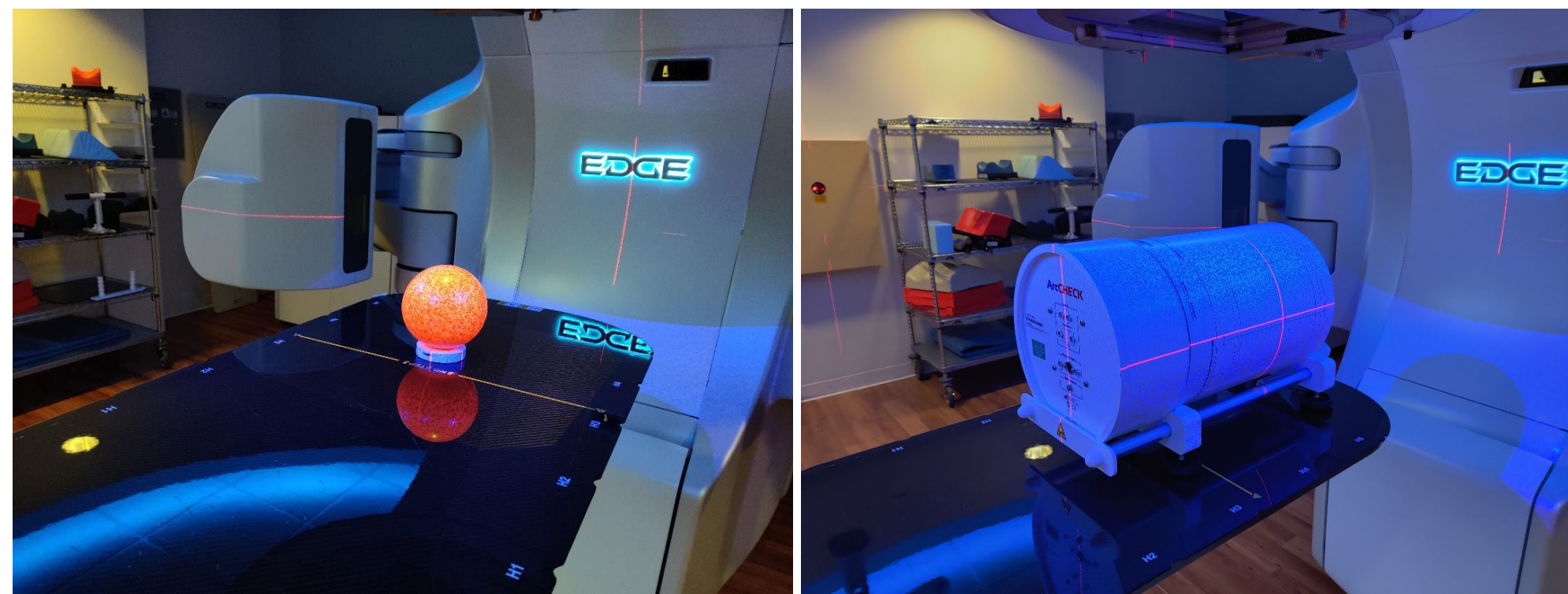
Figure 1. Spherical phantom (left) and cylindrical phantom (right) setups for breast and limb surface simulation. A red glossy spherical phantom (12-cm diameter) was positioned with its center of rotation aligned to the machine isocenter. Due to the phantom's isotropic symmetry, rotational tracking was evaluated only for the RTN (yaw) axis, as performance in PITCH and ROLL was assumed equivalent under rotational invariance.
