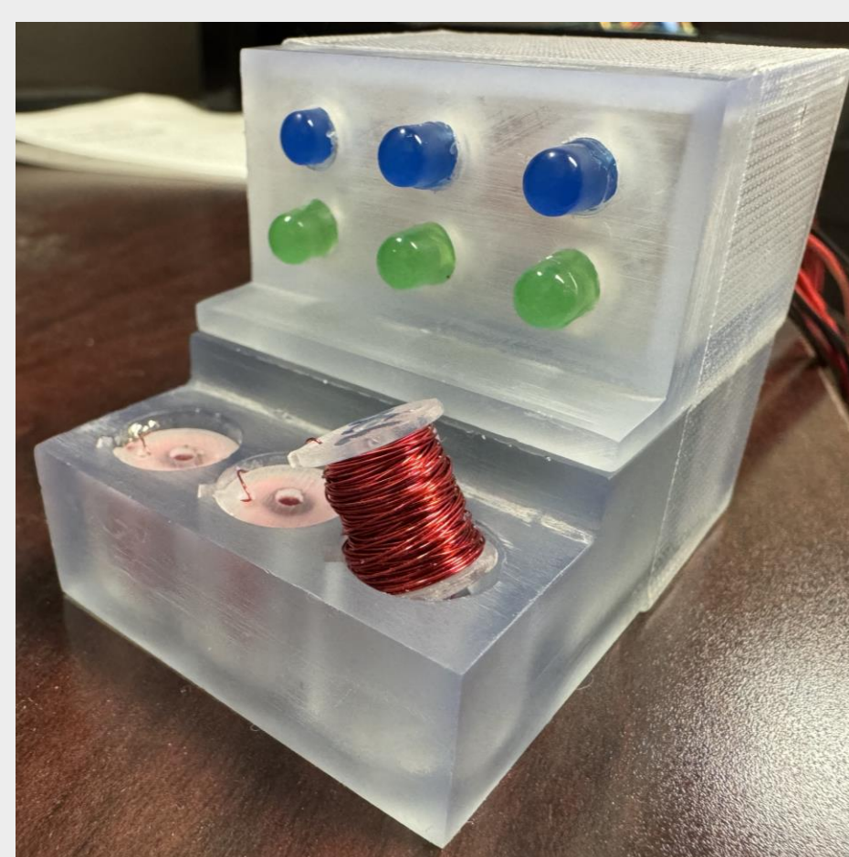
Figure 2. A photo of the safety device with an embedded solenoid exposed.
