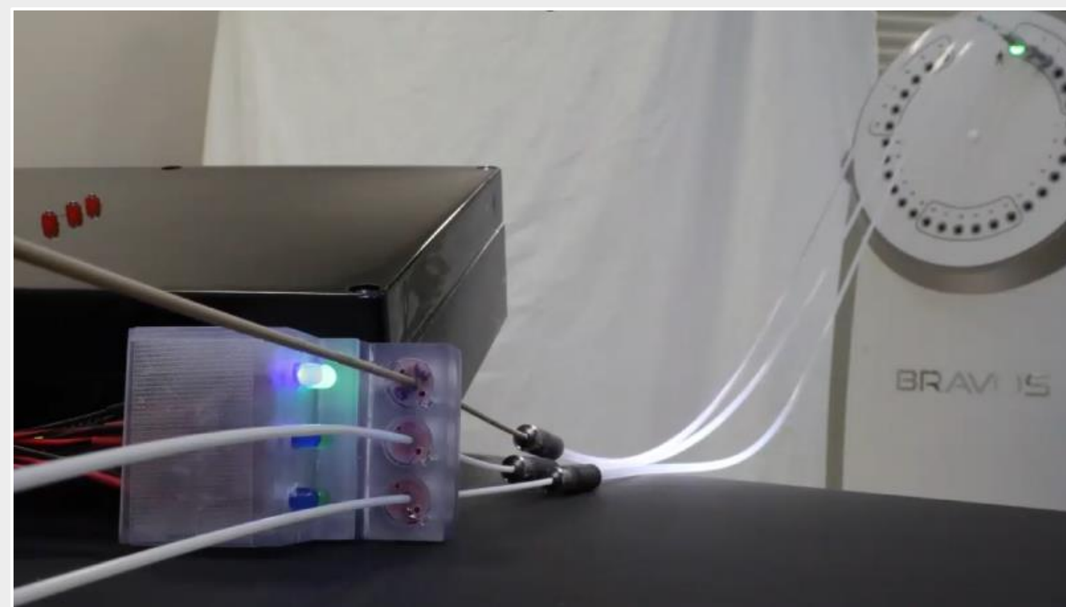
Figure 3. A photo of a trial where afterloader channel 1 is active. Both the blue and green LEDs are active on channel 1 indicating a correct channel connection
