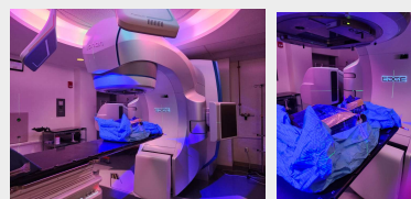
Fig 1. Anthropomorphic phantom with Dual Orthogonal kV Imaging and Thermal/Optical Surface Guidance.
