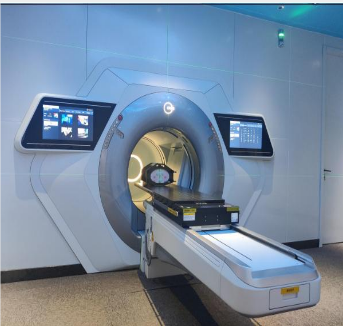
Fig 1: O-shaped TaiChiPro linear accelerator with intelligent couch shifting function.
