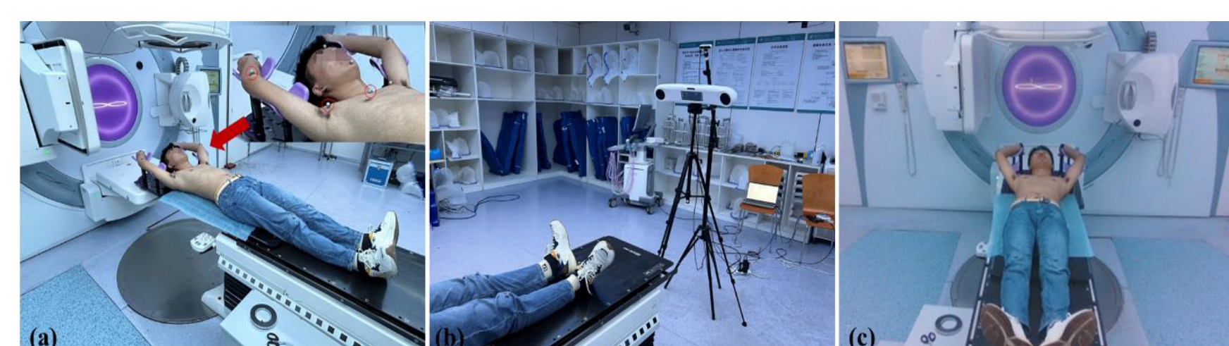
Figure 1. Radiotherapy-environment data acquisition setup: (a) placement of 17 motion-capture markers; (b) optical tracking and RGB camera configuration; and (c) representative RGB image.
