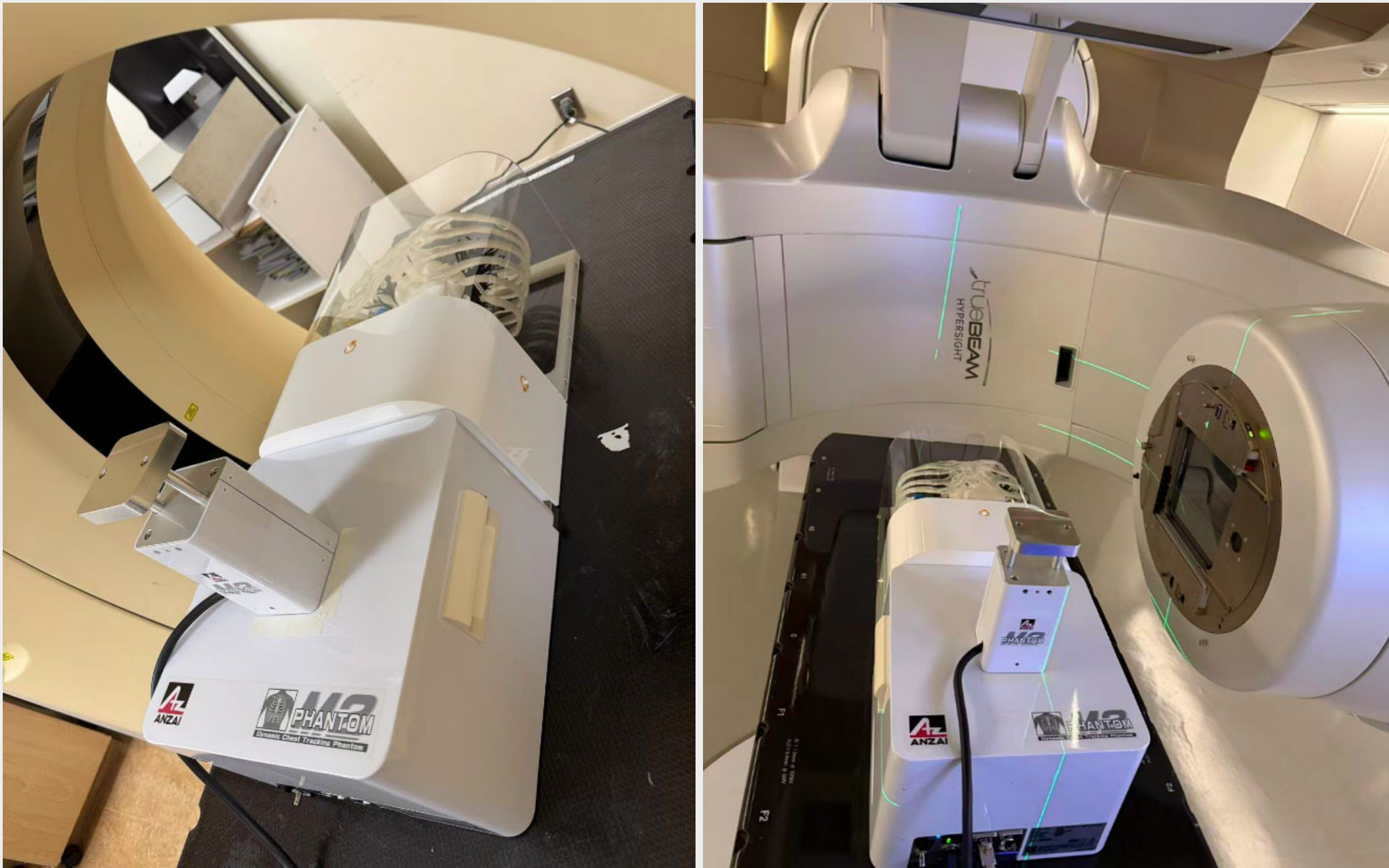
Figure 2. Phantom set up on (a) the Philips Big Bore CT couch for 4DCT (BBs for room laser alignment) and (b) the Varian TrueBeam couch.
