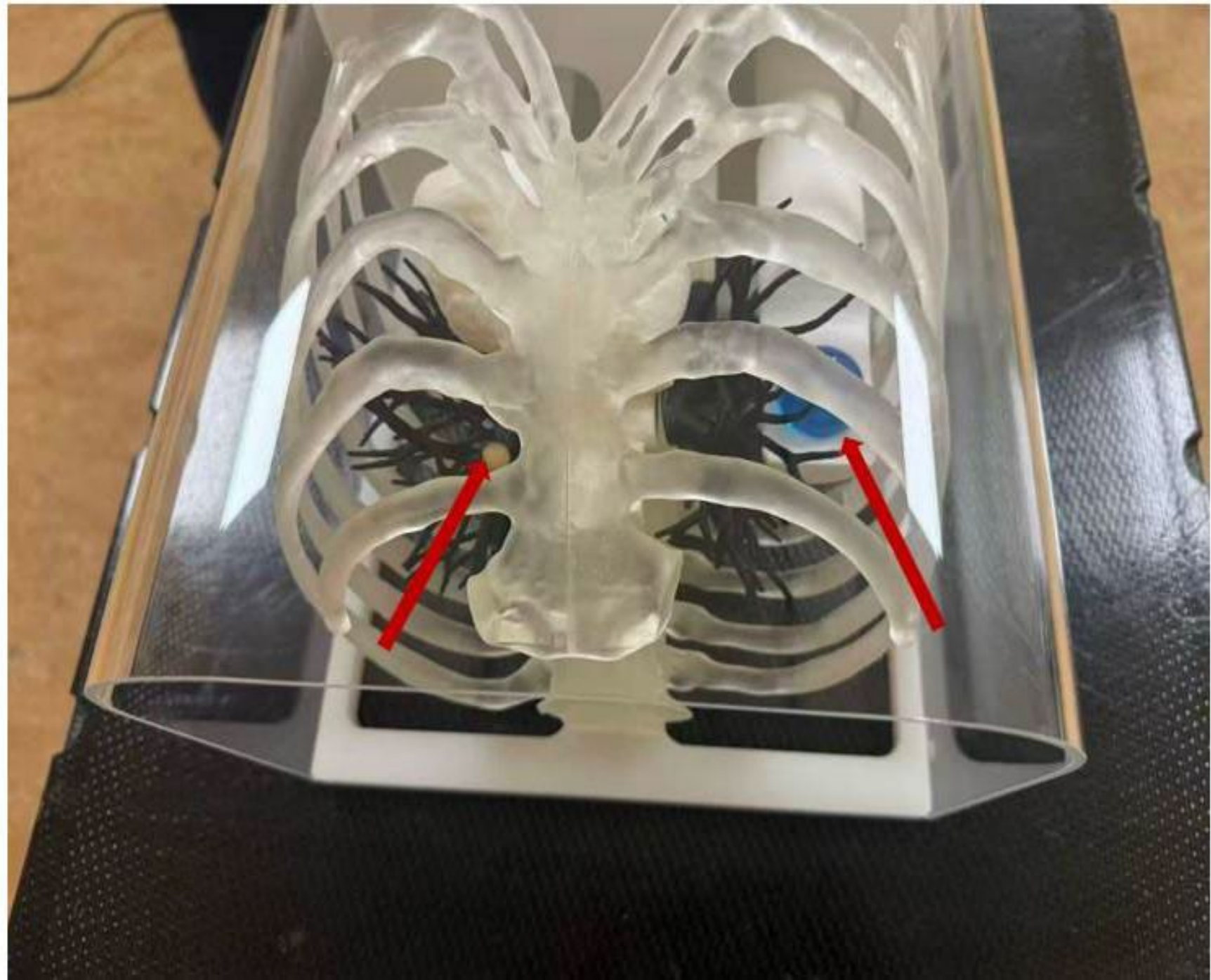
Figure 1. AZ-M2 dynamic chest motion phantom with independently moving tumor and vessel inserts.
