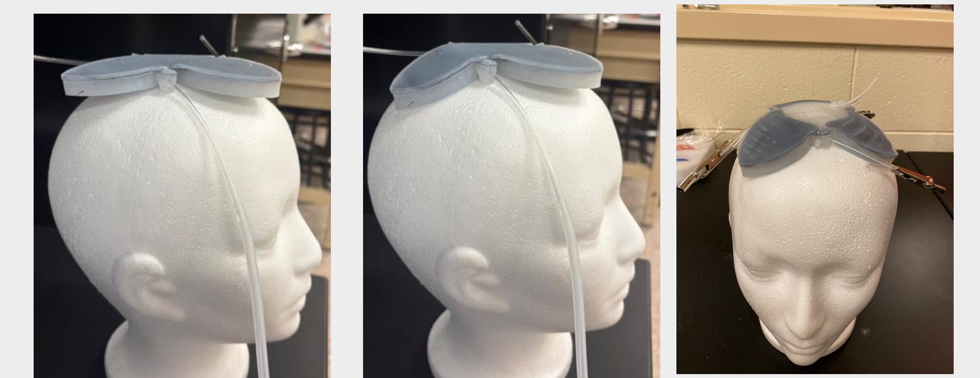
Figure 4. Example application, center uniform region with outer petal design as a first pass at mild suction.
