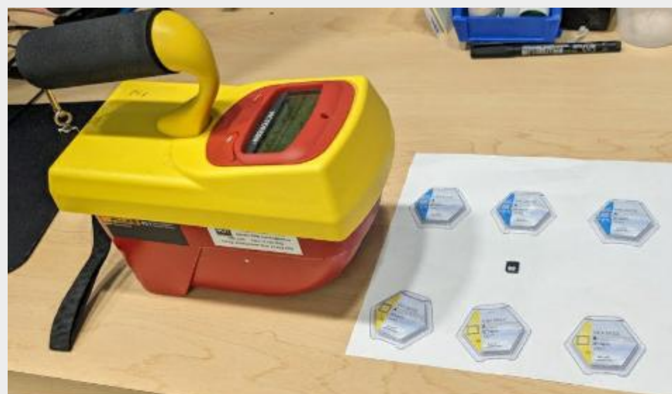
Figure 1 Dosimeter badges (along with survey meter and OSL chip) placed on a counter, for each exposure, at 3 meters away from isocentre, in the treatment room.
