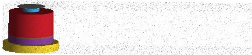
Figure 1. PTW 34013 ion chamber Model in EBrachy
