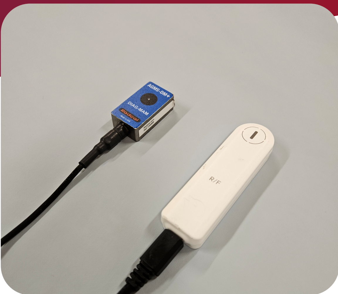
IBA Radcal AGMS-DM+ (left) and Raysafe X2 (right) solid-state dosimeters
